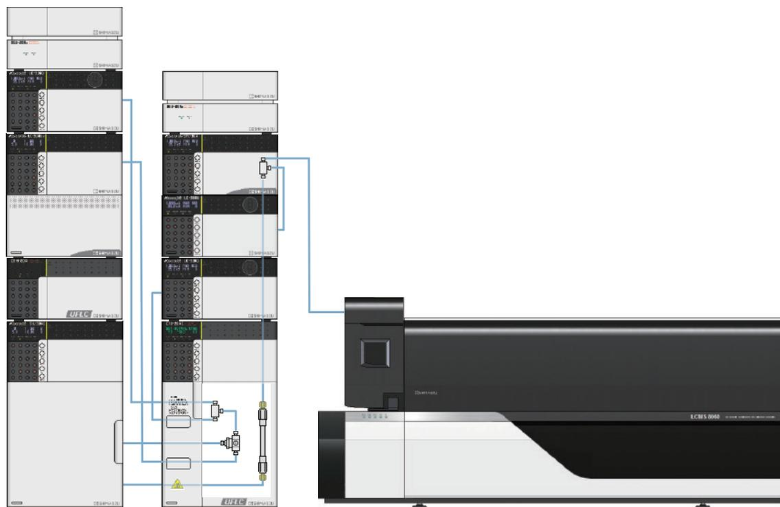
Figure 2: Setup of the SFC-MS/MS analytical system
