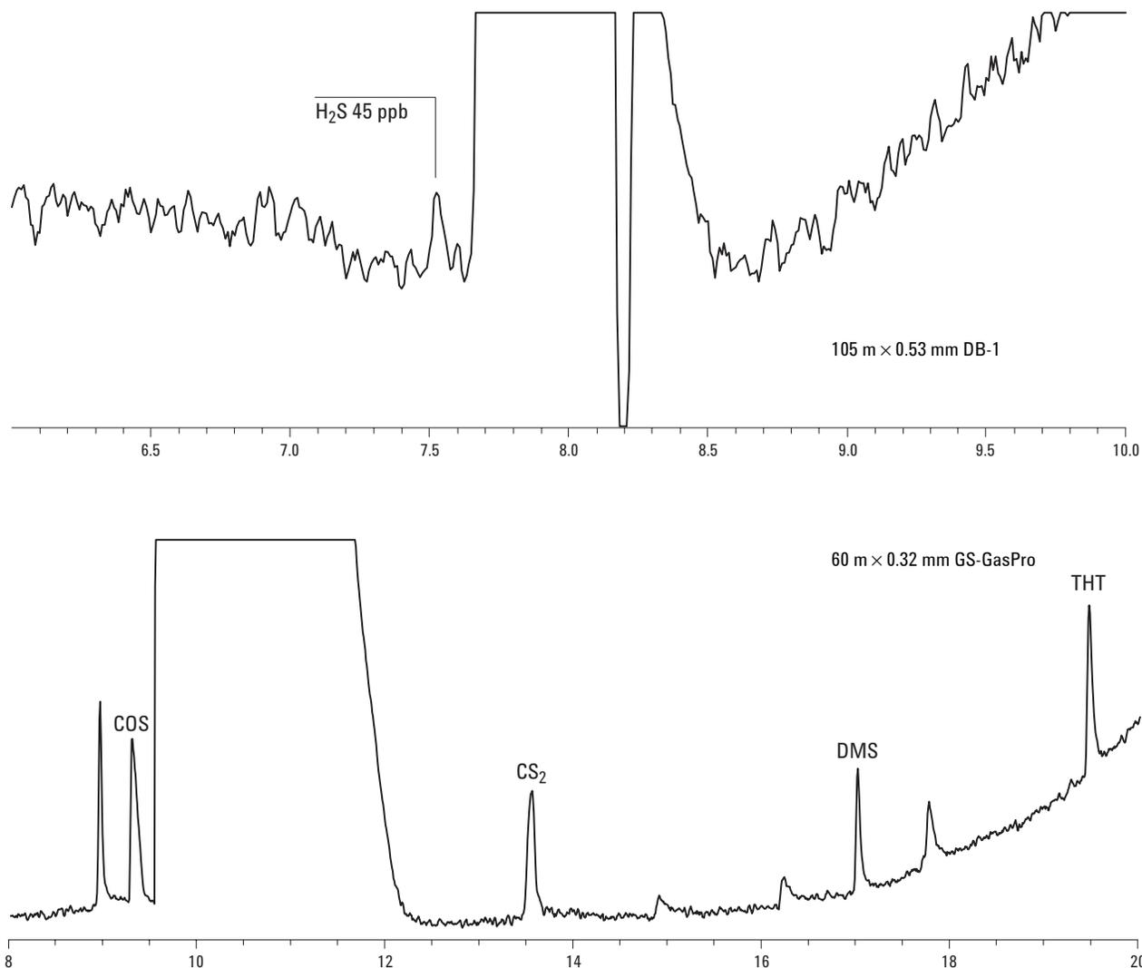
**Figure 6. Polymer-grade propylene blend containing 45 ppb (v/v) each of the eight sulfur compounds. Split ratio is 2:1. Top chromatogram: 105 m x 530  $\mu$ m DB-1 showing only H<sub>2</sub>S, bottom: 60 m GS-GasPro.**
