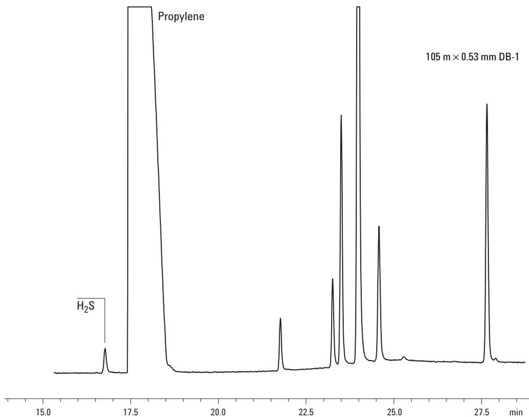
**Figure 7. Use of cryogenic oven temperatures for analysis of H<sub>2</sub>S (400 ppb) in propylene at 0.5:1 split.**
