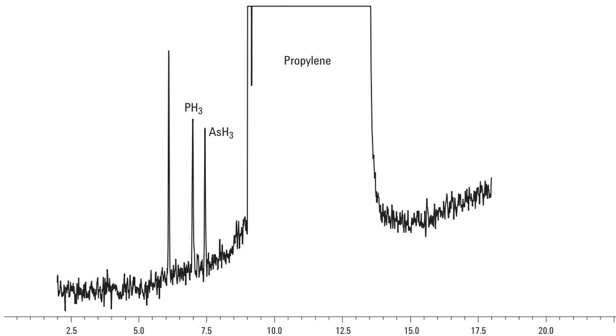
**Figure 9. Arsine optimized FPD flows. H<sub>2</sub>: 50 mL/min, air: 150 mL/min. 60 m × 0.32 mm GS-GasPro, 0.5 to 1 split. 90 ppb each of AsH<sub>3</sub> and PH<sub>3</sub>.**
