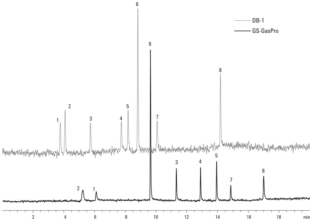
**Figure 3. The dual-column advantage. Sulfur mix at 90 ppb per component in helium. 1. H<sub>2</sub>S, 2. COS, 3. MeSH, 4. EtSH, 5. DMS, 6. CS<sub>2</sub>, 7. t-BuSH, 8. THT.**
