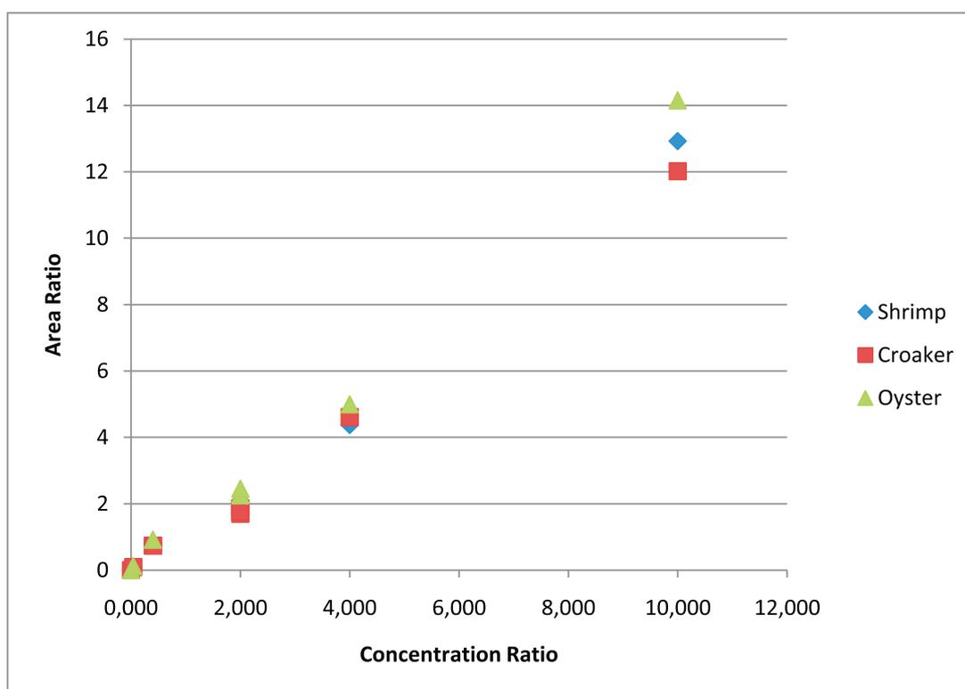
**Figure 1.** Pyrene Calibration Curves for Matrix Spikes.
