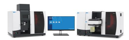
The Agilent AA Duo package allows you to run both your high and low concentration analytes at the same time. By controlling a dedicated flame and a dedicated furnace instrument from a single computer you can get simultaneous results from both.
