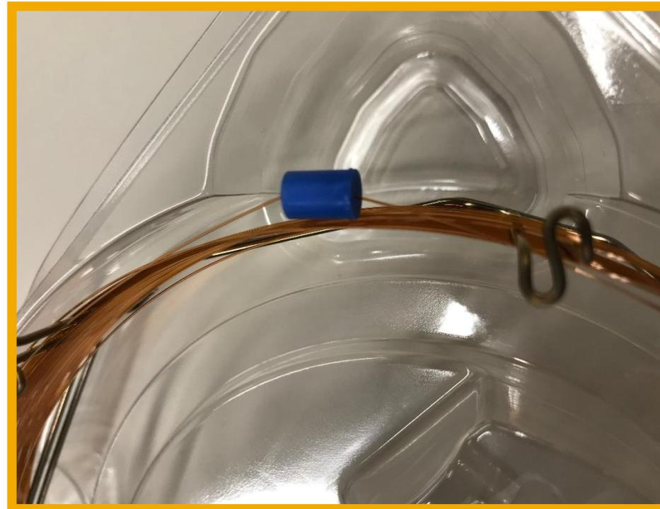
Column plug holds column ends together and protects against contamination. To put the column in storage, use this plug again or a piece of septa over the ends of the column.
