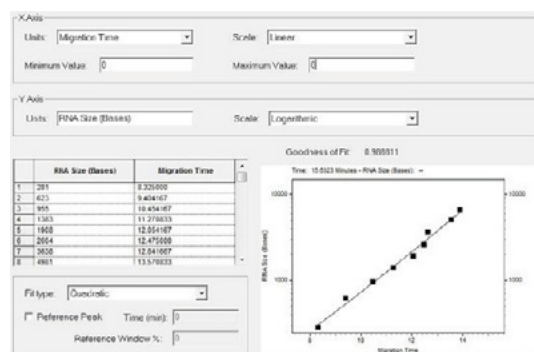
Figure 7. Calibration curve of log RNA Size in bases vs migration time of the Promega RNA ladder. R2 is 0.988811.
