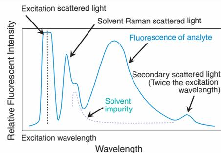
Fig. 2 Characteristics of Fluorescence Spectrum
