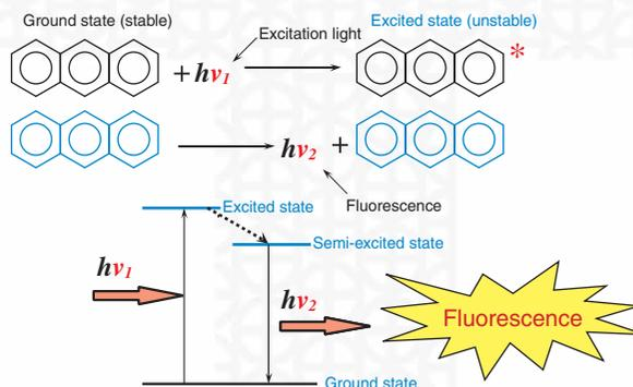
Fig. 1 Mechanism of Fluorescence from a Substance
