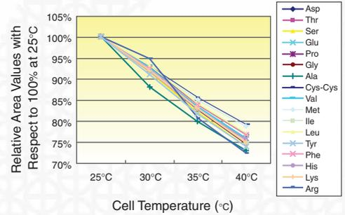
Fig. 7 Relative Area Values (%) at Each Temperature Assuming 100% at 25°C
