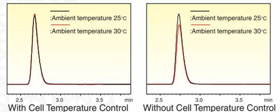
Fig. 9 Comparison of Chromatograms With and Without Cell Temperature Control
