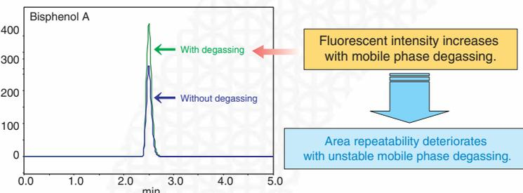
Fig. 5 Change in Peak Intensity due to Dissolved Oxygen in Mobile Phase
