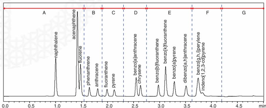
Fig. 15 Simultaneous High-Speed Analysis of 15 Polycyclic Aromatic Hydrocarbons
