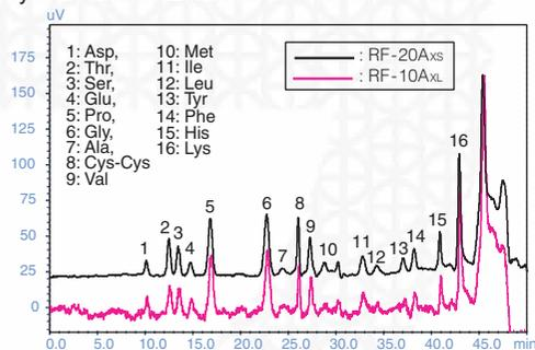
Fig. 16 Comparison of Amino Acid Analysis Using the RF-10AxL and RF-20Axs
