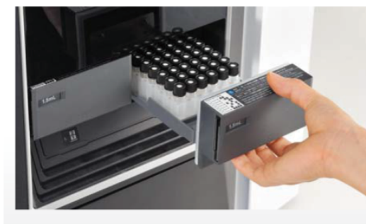
Fig. 2 Direct Access for Each Sample Rack
