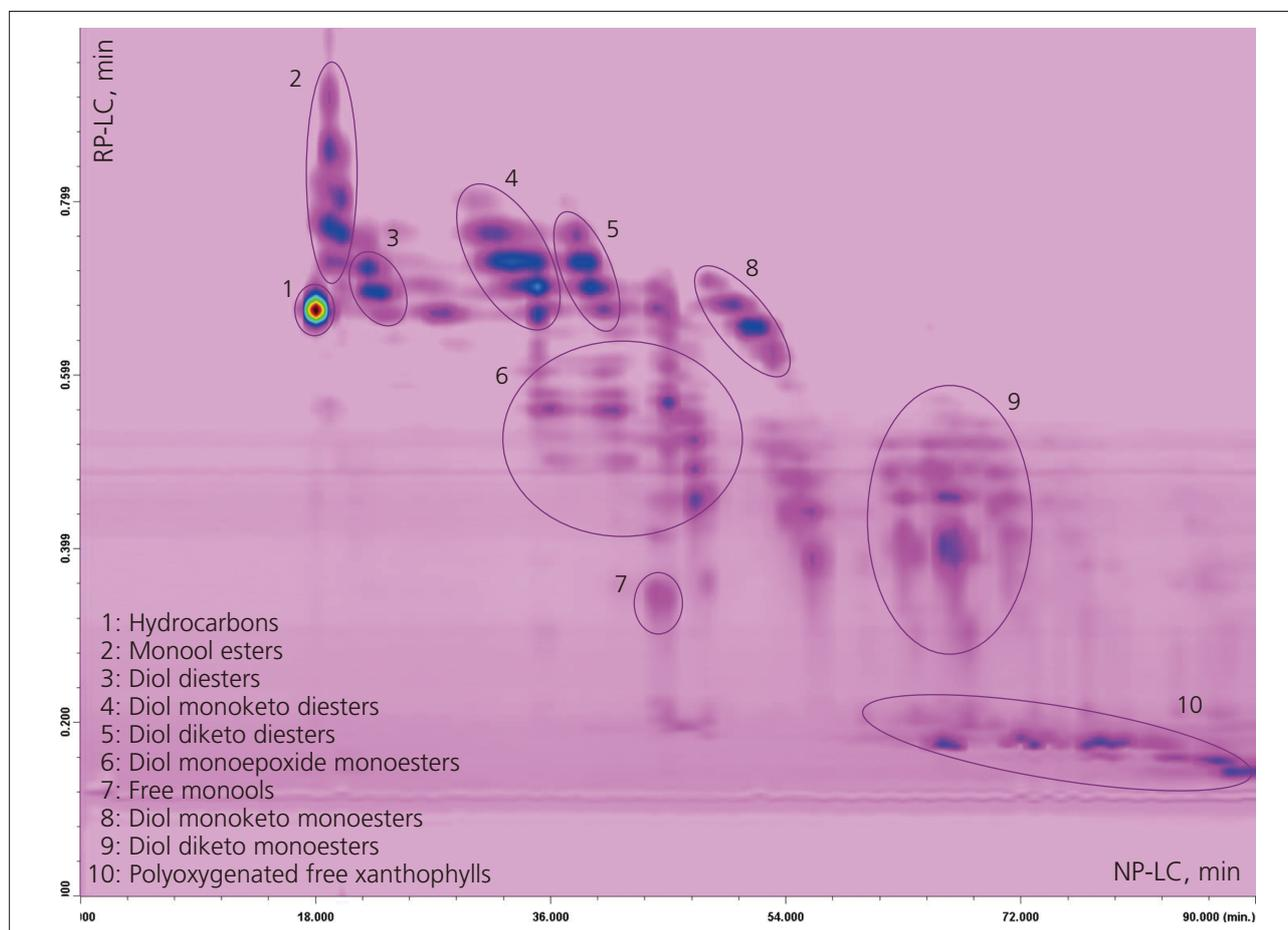
Fig. 1 2D Plot of Carotenoids Using ChromSquare Software
