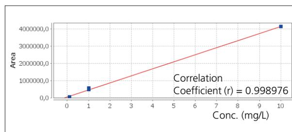
**Fig. 4 Linearity of Calibration Curve for  $\beta$ -Carotene**
