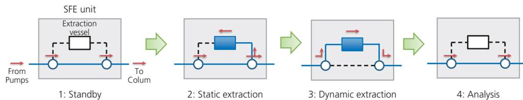
Figure 1. Flow diagrams of Nexera UC systems
