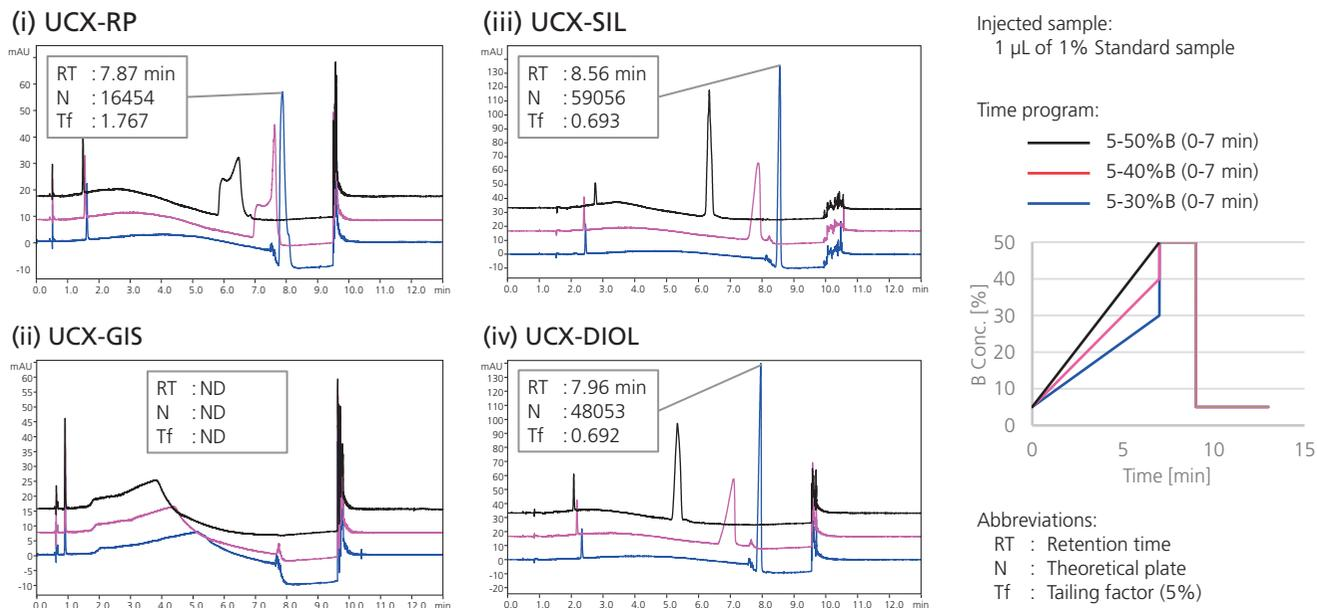
Figure 2. Comparison of columns for SFC analysis of standard detergent sample
