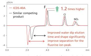
Fig. 4 Comparison of Chromatograms for Standard Anion Samples Resulting from Suppressor Differences
