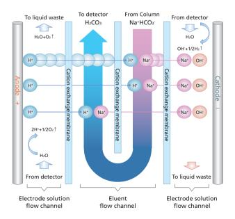
Fig. 3 Structure of the ICDS-40A and Suppressor Effect
