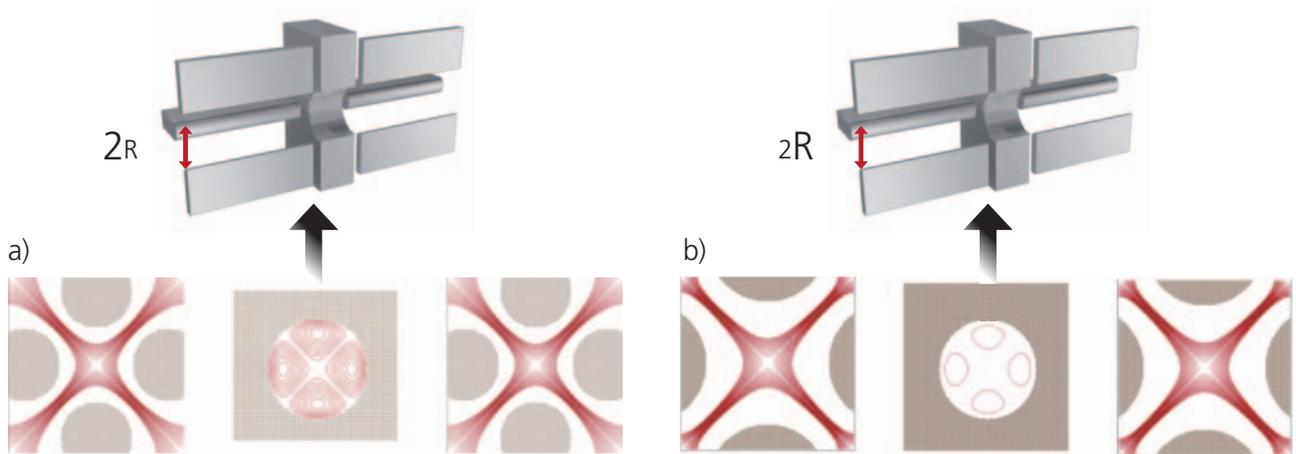
Fig. 4 Simulated fringing focusing field estimates of a) smaller R ion guides was found to be more effective than those of b) larger R. Therefore we have achieved higher sensitivity using smaller R ion guides.
