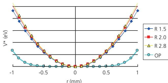
Fig. 3 Pseudo-potential of each tandem RF ion guide systems.
