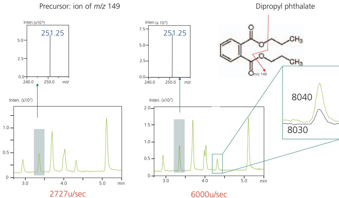
Fig. 6 Precursor ion scan of standard mixture sample of 8 phthalate esters.
