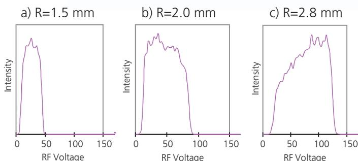
Fig. 2 The optimum operating RF voltage of quadrupole ion guides was acquired experimentally. The voltages were 27 V, 50 V and 100V for R= 1.5, 2.0 and 2.8 respectively.
