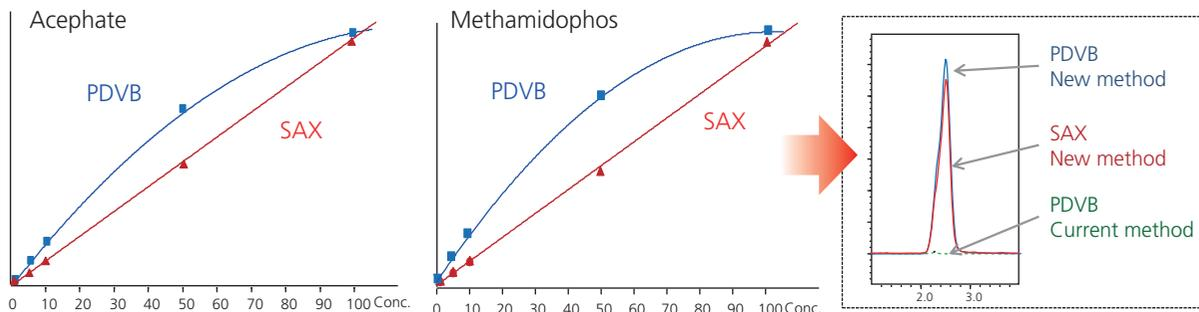
Fig. 8 Comparison of calibration curves and chromatograms (PDVB vs SAX)
