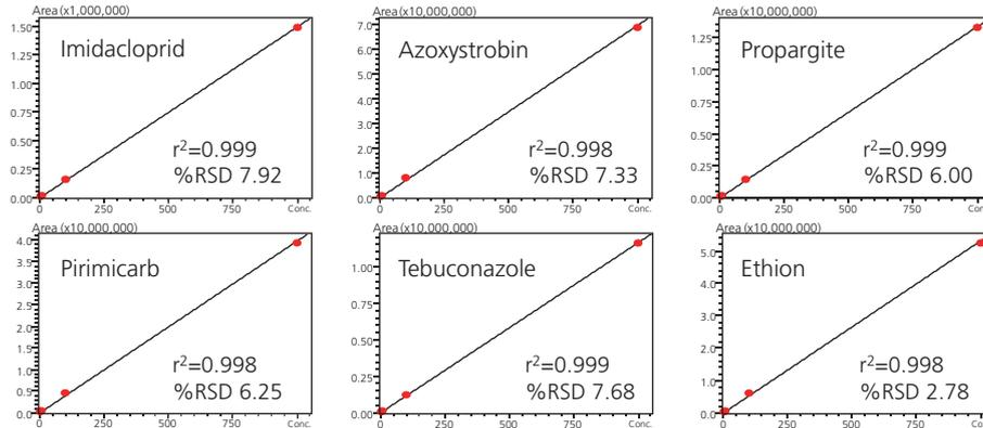
Fig. 4 Calibration curves of typical pesticides (5-1000 ppb)
