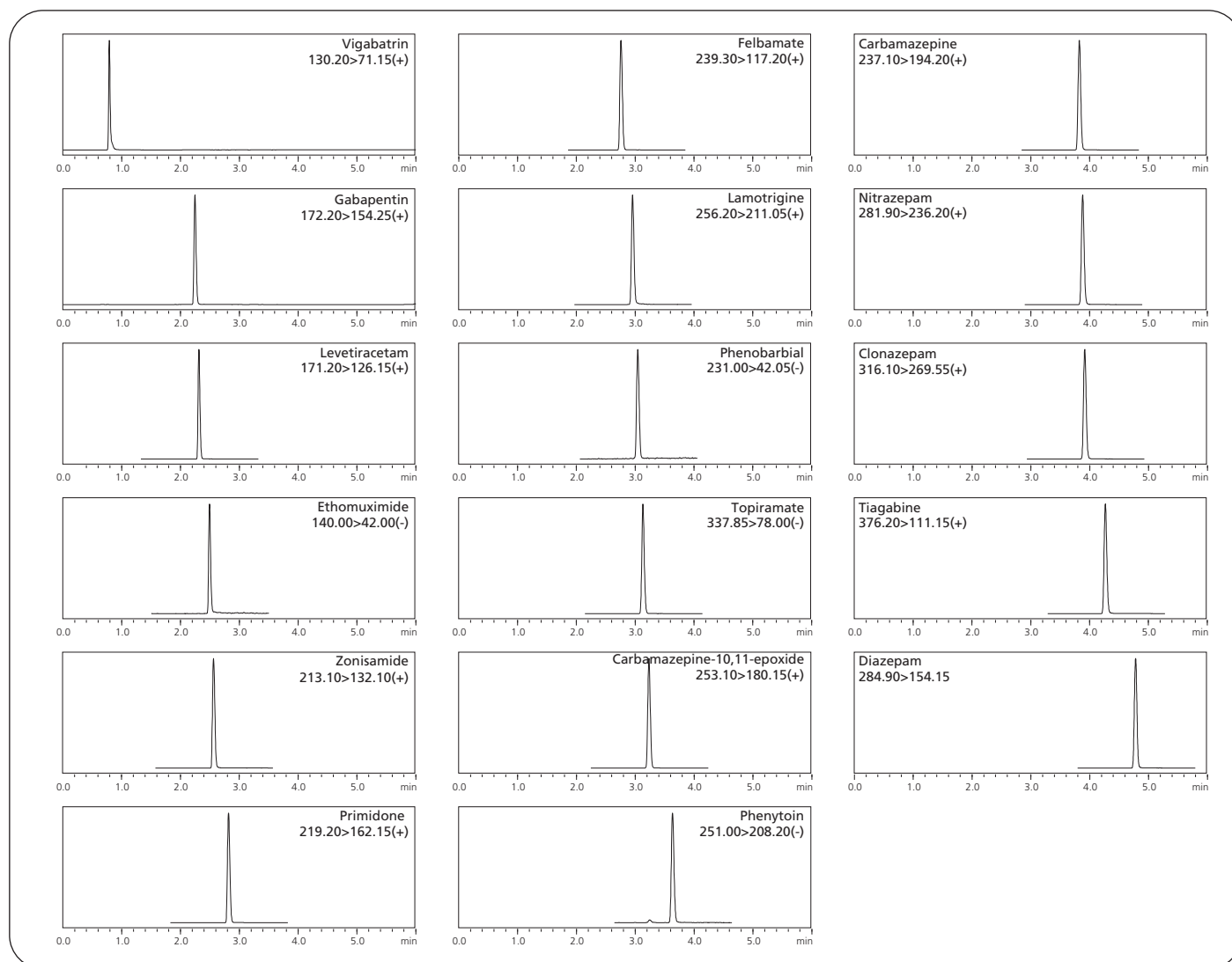
Figure. 4 Chromatogram of 17 AEDs calibration standards
