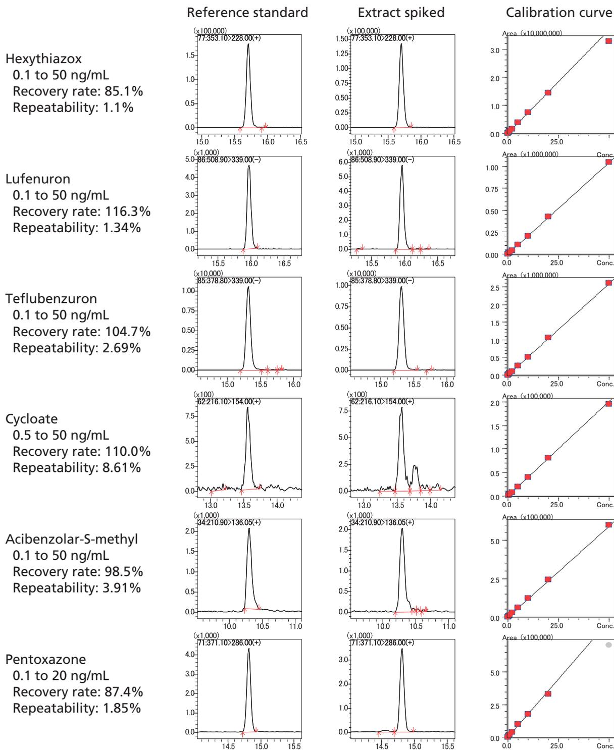
Figure 6. MRM chromatograms of reference standard 1 ng/mL, extract spiked with 1 ng/mL as final concentration with calibration curve.
