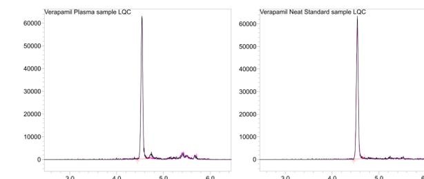
Figure 3 Chromatogram of Verapamil (MRM) in plasma spiked extracted sample and neat standard solution (LQC 1 ug/L)
