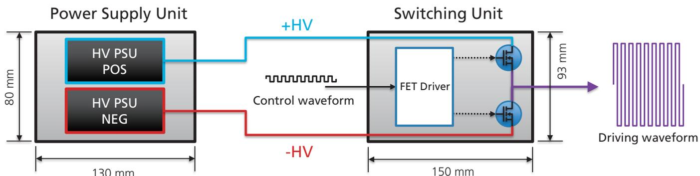
Figure 4 Diagram of the DIT driving unit
