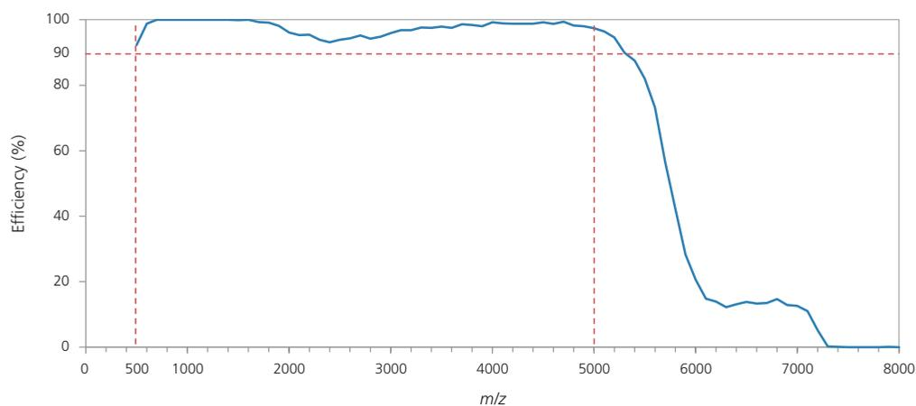
Figure 5 Simulation study on trapping efficiency by  $m/z$
