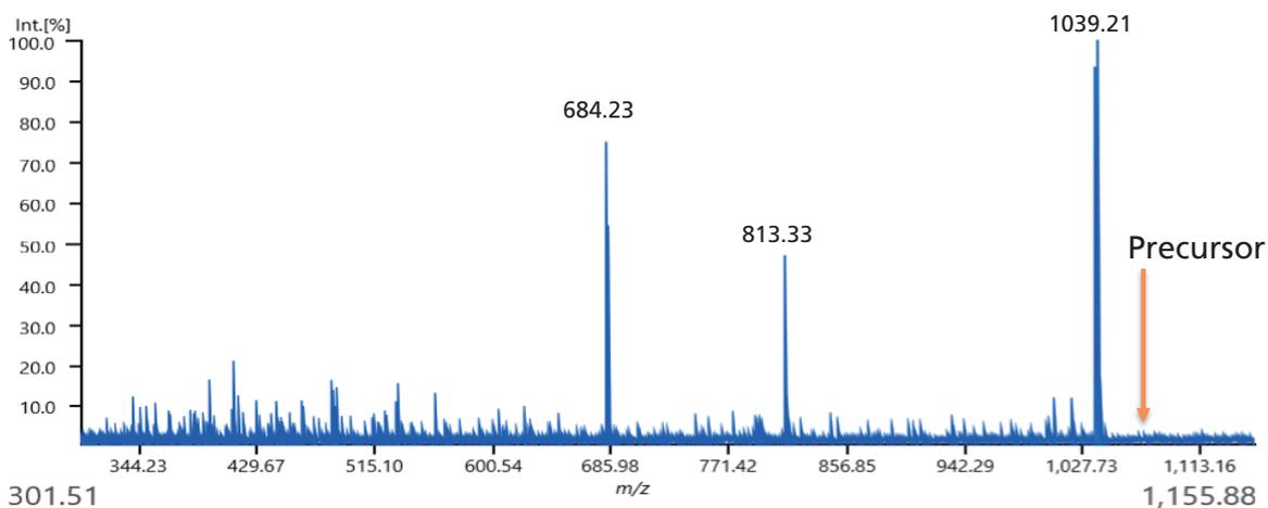
Figure 9 MS<sup>3</sup> Spectrum of the fragment ion peak of *m/z* 1056 from 100 fmol of Glu-1-Fibrinopeptide B
