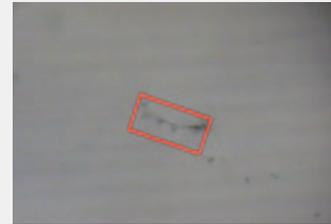
Microscope Photograph of Foreign Substance on Film
