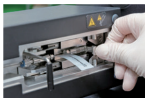
Place the column in the UF-Link mechanism in the oven.
