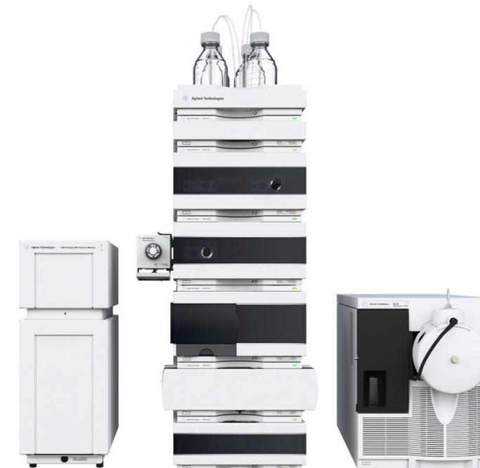
The Agilent 1260 Infinity hybrid SFC/UHPLC system combined with single quadrupole mass spectrometry detection is capable of performing both supercritical fluid chromatography (SFC) and ultrahigh performance liquid chromatography (UHPLC) by switching automatically between the two techniques.
