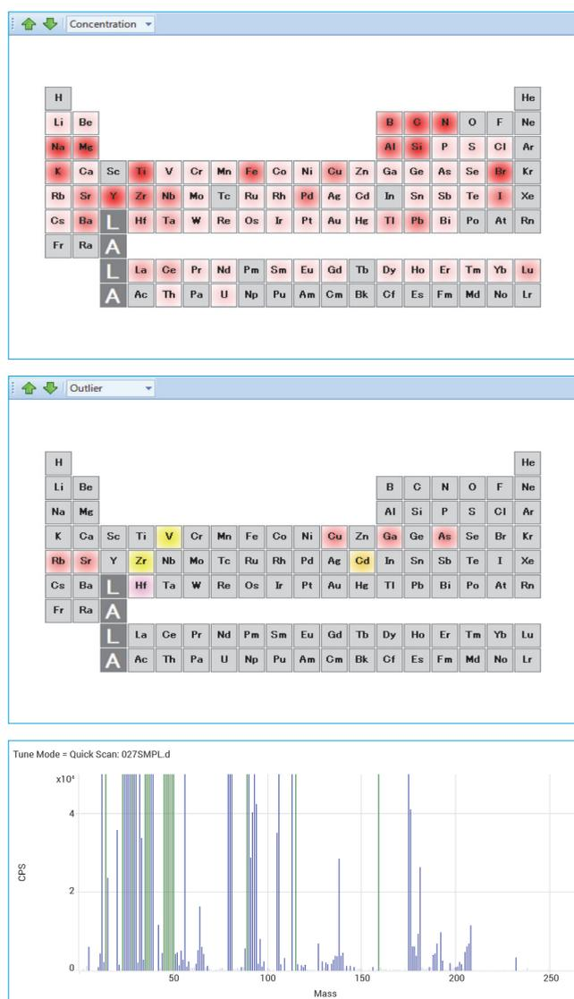
**Figure 2.** Top and middle: ICP-MS MassHunter IntelliQuant concentration heat map and outlier flags indicating possible spectral overlap. Bottom: Quick Scan full mass spectrum enables identification and confirmation of semiquantitative results for uncalibrated elements.
