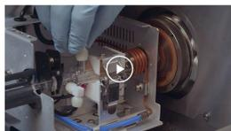
Eliminate plasma ignition problems and maintain optimal performance. Learn how to inspect the torch, bonnet, shield plate, and RF coil. We'll also show you how to clean the torch.
