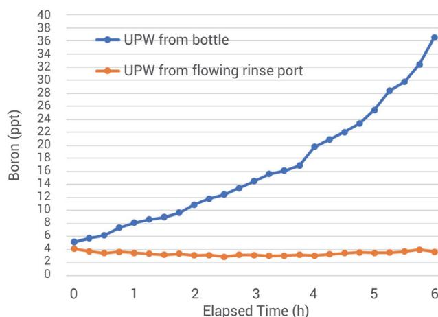
**Figure 2.** Boron blank level (ppt) in UPW from container (blue) and from flowing rinse port (orange).
