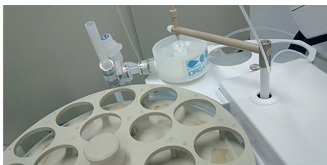
**Figure 1.** Agilent I-AS autosampler with Organo UPW flowing rinse port system.
