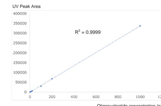
Figure 5. Calibration curve of the 21-mer oligonucleotide showing linearity over three orders of magnitude. Peak areas obtained from the TUV detector were plotted against a wide range of oligonucleotide concentrations, including 0.5, 1, 5, 10, 20, 100, 200 and 1000 nM. Excellent signal linearity was obtained for this assay, indicating that very low oligonucleotide concentrations can be recovered completely from a very inert LC system that does not interact in any way with the analyte.
