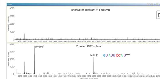
Figure 2. Ion pairing reversed-phase (IP RP) ESI-MS spectra recorded for: (A) the most abundant sample component, the 21-mer heavily modified oligonucleotide; (B) the least abundant sample component, an 11-mer oligonucleotide impurity (see Table I for its sequence), present at 0.18% according to the UV peak area measurement.
