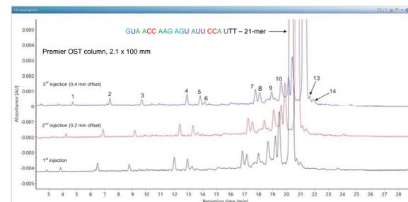
Figure 1C. Three replicates injections performed on the ACQUITY Premier OST column. For better clarity, the red and blue traces are offset by +0.2 min from the previous trace.
