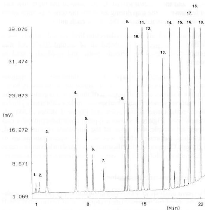
**Figure 4.** Ethane to isoprene, from 27 component VOC standard cylinder. 1. Ethane, 2. Ethene, 3. Propane, 4. Propene, 5. 2-Methylpropane, 6. Ethyne, 7. n-Butane, 8. *trans*-2-Butene, 9. 1-Butene, 10. *cis*-2-Butene, 11. 2-Methylbutane, 12. n-Pentane, 13. 1,3-Butadiene, 14. *trans*-2-pentene, 15. *cis*-2-Pentene, 16. 2-Methyl pentane, 17. 3-Methylpentane, 18. n-Hexane, 19. Isoprene.
