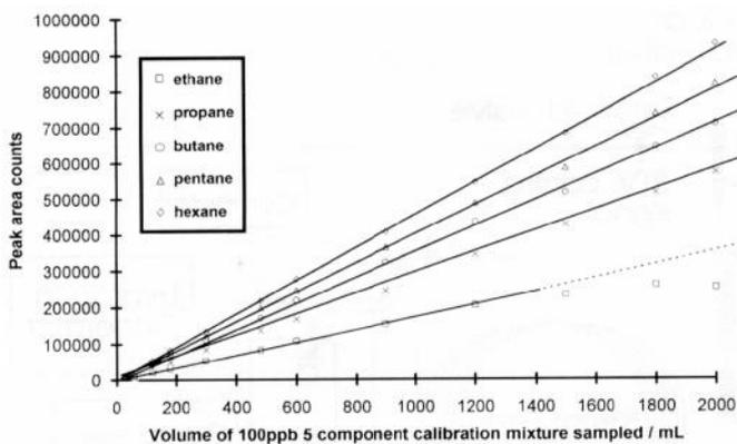
**Figure 2.** Sampling loading curves @  $-10^\circ\text{C}$ .
