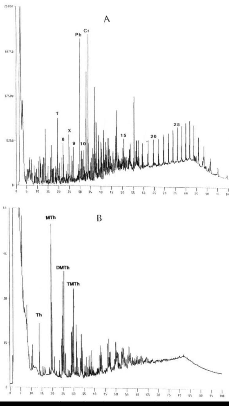
Fig. 8. Pyrolysis at 530°C of the Malaysian source rock sample. Type III kerogen: aromatic with high landplant input. Sample intake = 1.6 mg; pyrolysis time=2 min, AED. (A) Carbon signal (193 nm); (B) sulphur signal (181 nm). Numbers are carbon numbers of alkanes/alkenes; T=toluene, X=xylene, Ph=phenol and Cr=cresols.
