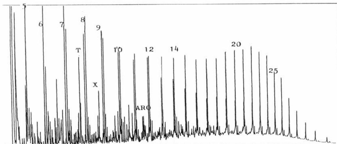
Fig. 9. Pyrogram of Australian source rock (as in Fig. 6A) obtained with a CDS Pyroprobe 100 pyrolyzer. Sample intake=24.9 mg; pyrolysis time=20 s, pyrolysis temperature=530°C, FID. For peak identification, see Fig. 6A.
