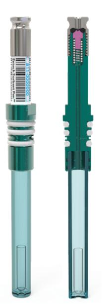
**Glass Sorbent Pen** (GSP) for Direct Thermal Desorption
