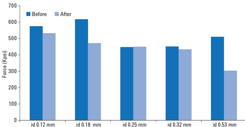
Figure 7. Strength of Agilent tubing before and after lifetime testing for 144 hours exposure at 360 °C.
