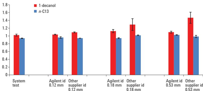
Figure 3. Asymmetry (measured at 10% peak height) of 1-decanol when using Agilent or other supplier deactivated fused silica tubing, compared to system test. Duplicate tubing was tested.
