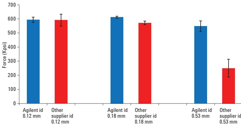
Figure 6. Strength test of Agilent and other supplier tubing at different internal diameters.
