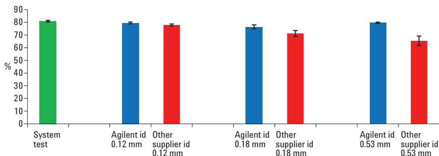
Figure 4. Relative recoveries (compared to *n*-tridecane) of 1-decanol when using Agilent or other supplier deactivated fused silica tubing, compared to system test. Duplicate tubing was tested.
