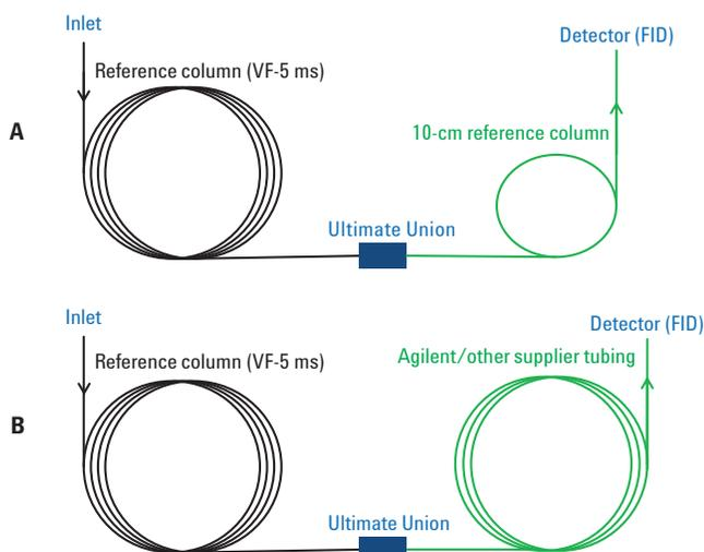
Figure 1. The tandem-column setup of system test (A) and Agilent/other supplier tubing test (B).
