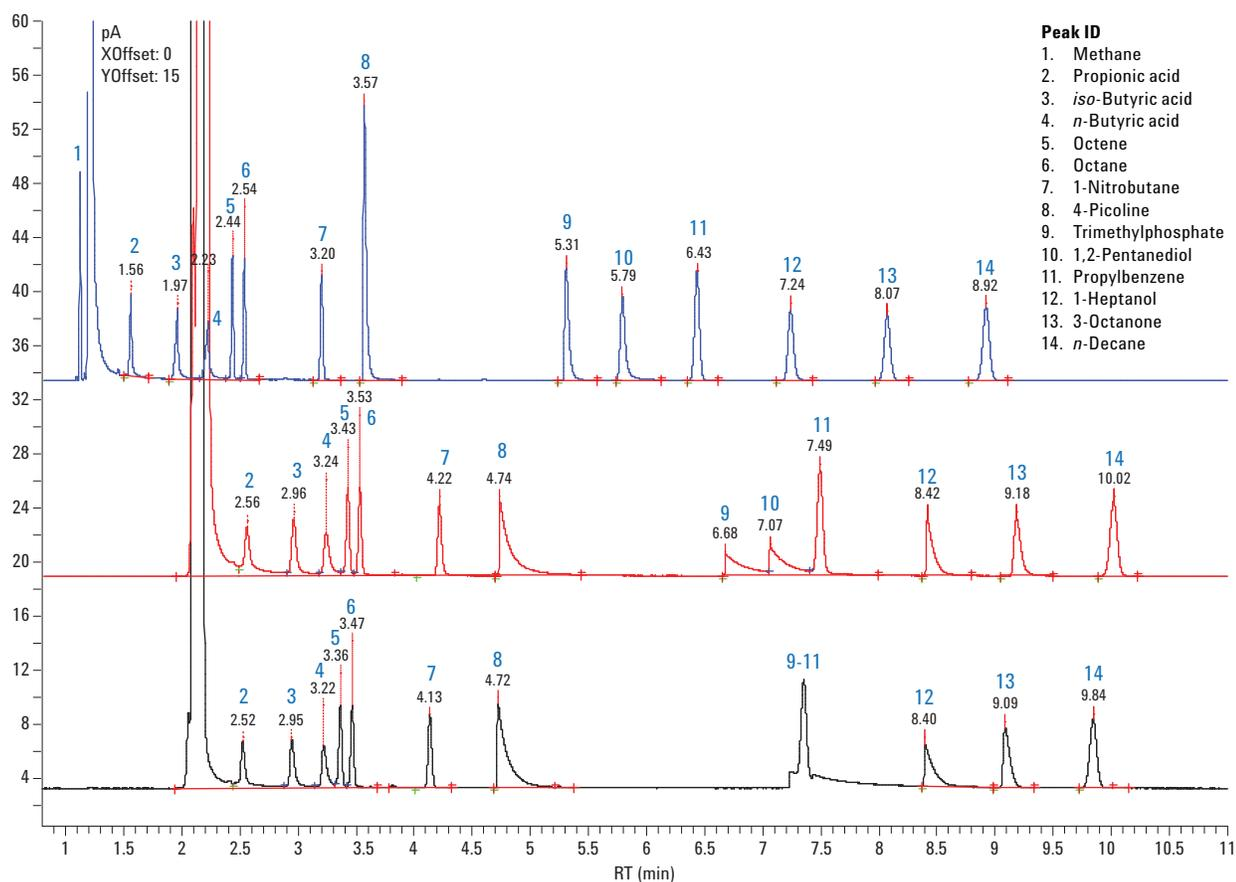
Figure 5. Comparison of different types of tubing, 6 m × 0.53 mm, using Very Inert Mix 2. Method as for Figure 2.
