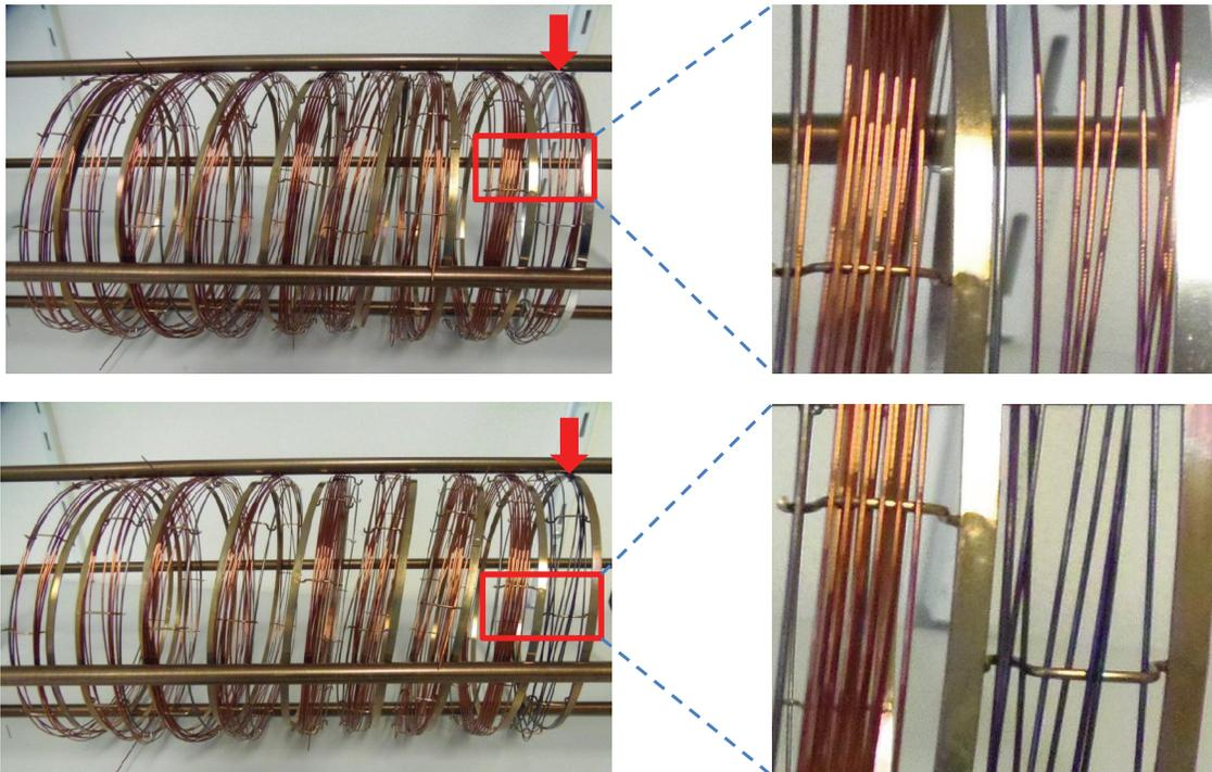
Figure 8. Eight Agilent fused silica tubes (left) and a fused silica tube from another supplier (right) before (top image) and after (bottom image) a temperature stability test at 360 °C over 72 hours.
