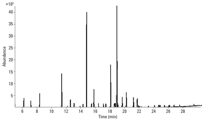
Figure 1. Representative chromatogram for analysis of the GLC Reference Standard GLC-603 using the Agilent 5973 Series GC/MSD.
