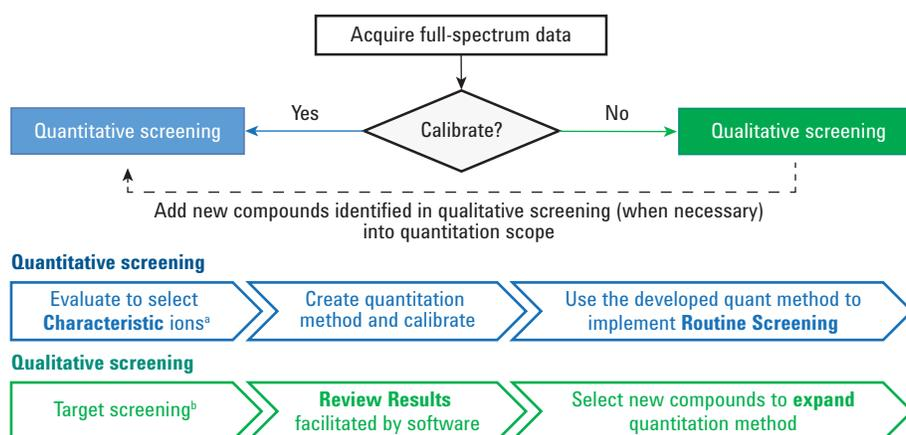
Figure 2. Workflow for quantitative and qualitative screening. <sup>a</sup>Evaluate is only applied to the method development stage with curated accurate mass spectra from the PCDL as an input for ion selection (a subset of compounds with standards for calibration). <sup>b</sup>Suspect screening against a PCDL subset including compounds without authentic standards.
