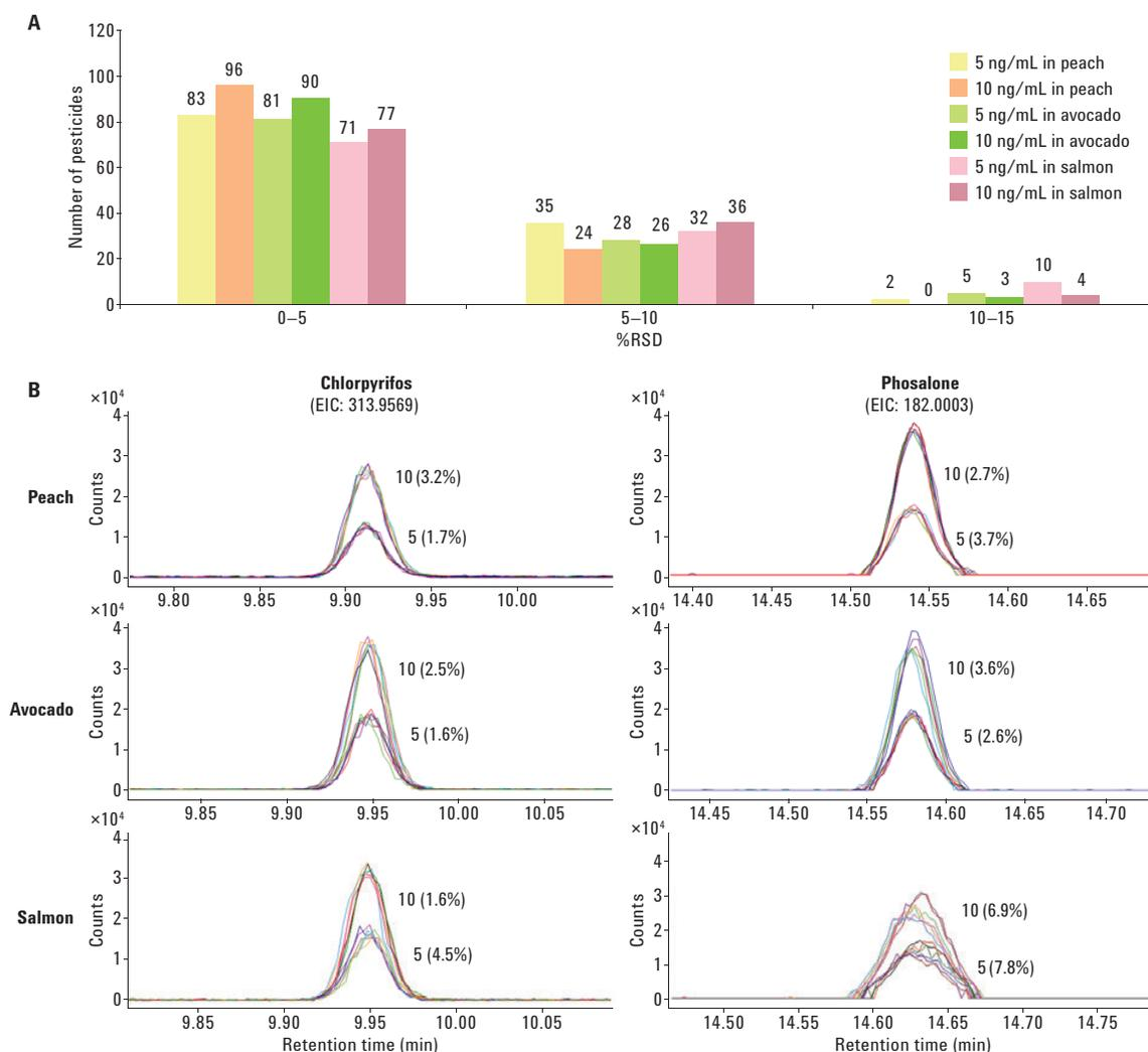
Figure 5. Response RSD% of pesticides in food matrices (A) and EICs of example compounds (B) from six replicate injections. EICs were extracted with a window of  $\pm 25$  ppm. Numbers inserted in example EICs follow the format: concentration with the unit of ng/mL and (%RSD).
