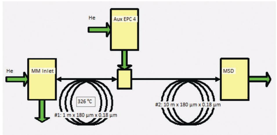
**Figure 2.** Backflush setup.
