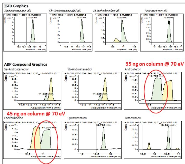
Figure 5A. The endogenous steroids androsterone and etiocholanolone may be present in urine at high concentrations, resulting in chromatographically overloaded, saturated peaks, hindering the initial testing procedure (screening).
