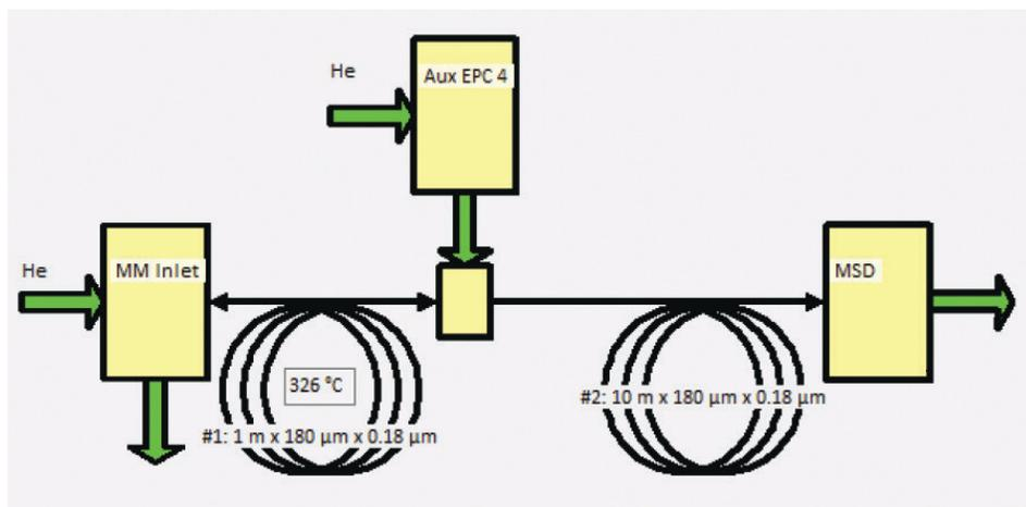
**Figure 2.** Backflush setup.
