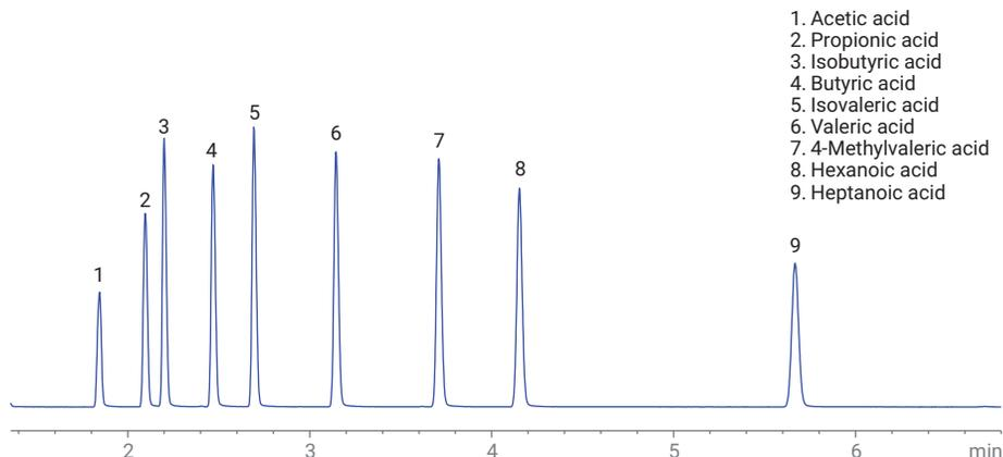
**Figure 1.** GC/FID chromatogram of a mixture of C2–C7 free fatty acids in water on a 30 m  $\times$  0.25 mm id, 0.25  $\mu\text{m}$  J&W DB-FATWAX Ultra Inert column (conditions listed in Table 2).
