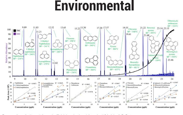
Sample: 0.5 – 10 ppb PAH mix in 10 mL 5% Na2SO4 **VASE:** Tenax TA (35/60) HSP, 16 h, 55°C, 150 rpm TD: 60 sec 200°C Preheat, 3 min 325°C Desorb, 18 min 300°C Bake-out GC-MS: DB-5MS (30m×0.25mm×0.5µm), Thermo TRACE 1310 ISQ
