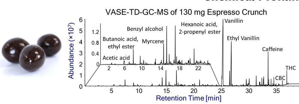
TD: 60 sec 175°C Preheat. 3 min 225°C Desorb. 30 min 300°C Bake-VASE: Tenax TA (35/60) HSP, 16 h, 70°C, 120 rpm GC-MS: DB-5MS (30m×0.25mm×0.5µm), Agilent 7890B/5977A
