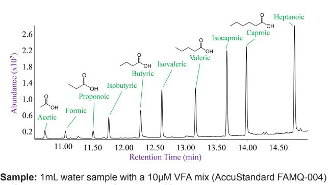
VASE: Tenax TA (35/60) HSP, 16 h, 35°C, 250 rpm **TD:** 120 sec 200°C Preheat, 3 min 260°C Desorb, 10 min 275°C Bake-out **GC-MS:** DB-WAX (60mx0.32mmx0.5µm), 20:1 Split, Agilent 7890A/5975C
