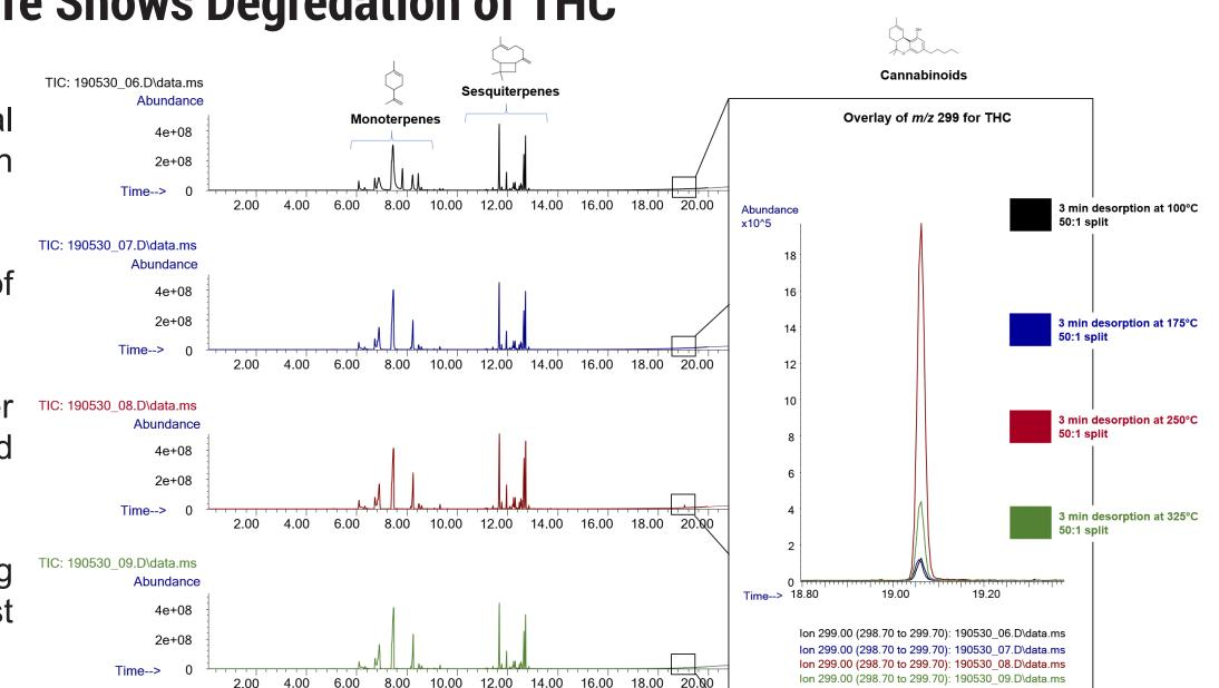
The aim of using the Trace Procedure for cannabis analysis is to split highly abundant volatile terpenes while allowing the cannabinoids to become trapped on Column 1 to enhance detection of these lower volatility compounds after a short extraction.
