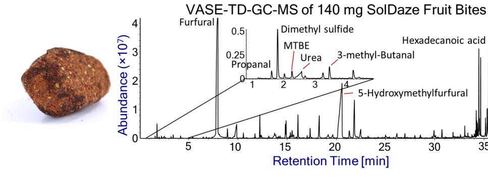
Sample: 140 mg fruit bite smudg VASE: Tenax TA (35/60) HSP, 16 h, 70°C, 120 rpm GC-MS: DB-5MS (30m×0.25mm×0.5µm), Agilent 7890B/5977A
