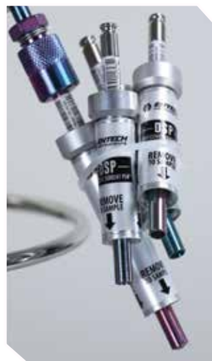
Fig 2 - 3 DSP samplers placed in close proximity to ASP sampler to compare sampling rates.
