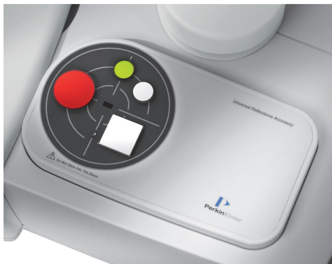
Figure 13. The Universal Reflectance Accessory (URA) fitted into a LAMBDA 950. The URA is a programmable motorized absolute reflectance with an angle range of 8-68 degrees.
