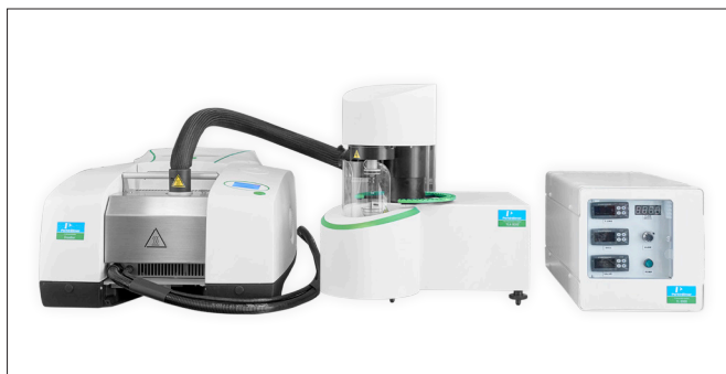
Figure 1. The TL 8000 transfer line couples a Frontier FT-IR to a TGA 8000.
