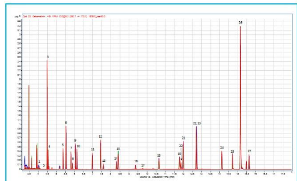
Figure 3. Overlaid chromatograms demonstrate the chromatographic consistency after calibration (blue), after completing an additional 60 matrix injections with black tea (red), and after guard chip replacement on the Intuvo system (green).
