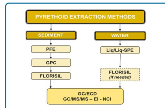
Figure1: A flow diagram of the sample preparative procedure shows the differences between water and sediment. PFE is an abbreviation for Pressurized Fluid Extraction and GPC is an abbreviation for Gel Permeation Chromatography.
