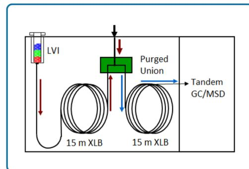
Figure 2: Tandem GC/MS system configuration with mid-column back flushing.
