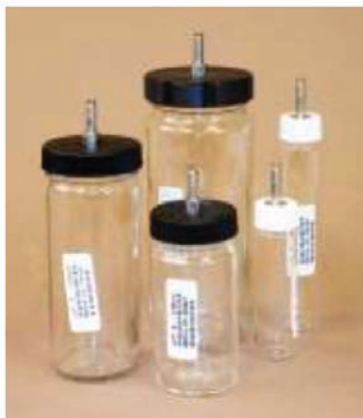
Figure 1 Vacuum tight vials ranging from 40 to 1000mLs utilize a septum-less interface that typically yields leak rates of less than 2 \times 10^{-8} cc/sec, making them appropriate for both vacuum extraction and Large Volume Static Headspace techniques.
