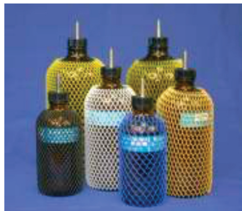
Figure 2 Bottle-Vac samplers can be used for both gas-phase and liquid/ solid sampling. Liquid samples with minimal suspended particulates can be injected directly through the Micro QT septum-less interface into a pre-evacuated bottle using a blunt end 16 gauge needle.
