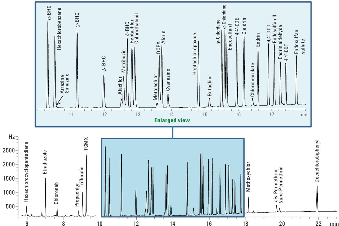
Figure 4. Enlarged section of the GC/ $\mu$ ECD chromatogram of a 10 ng/mL chlorinated pesticide standard analyzed on an Agilent J&W DB-XLB 30 m  $\times$  0.32 mm, 0.5  $\mu$ m column. The chromatographic conditions are listed in Table 1.
