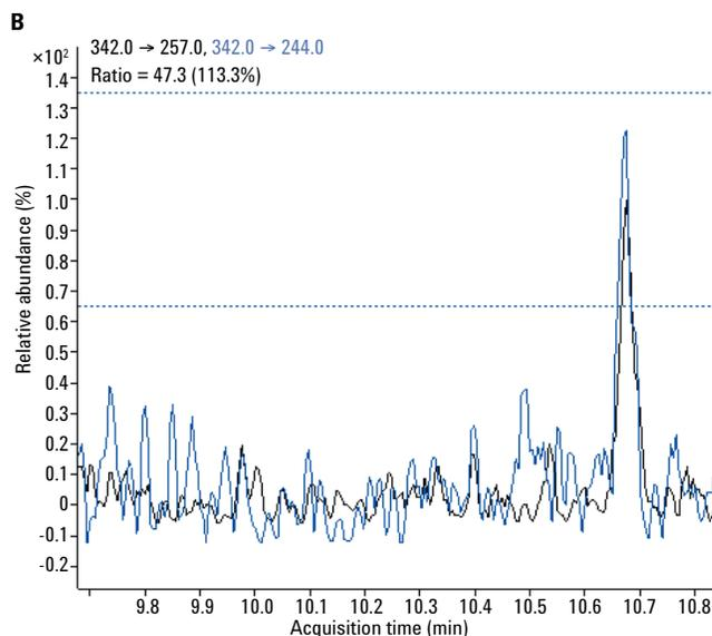
Figure 1. 1.0 ng/mL E1. **A** shows the quantitative SRM 342 → 257. **B** shows the qualitative transition 342 → 244. The dotted lines in **B** represent the allowable uncertainty for qualifier ratio. Noise region for S/N calculation is 10.4 to 10.6 minutes.
