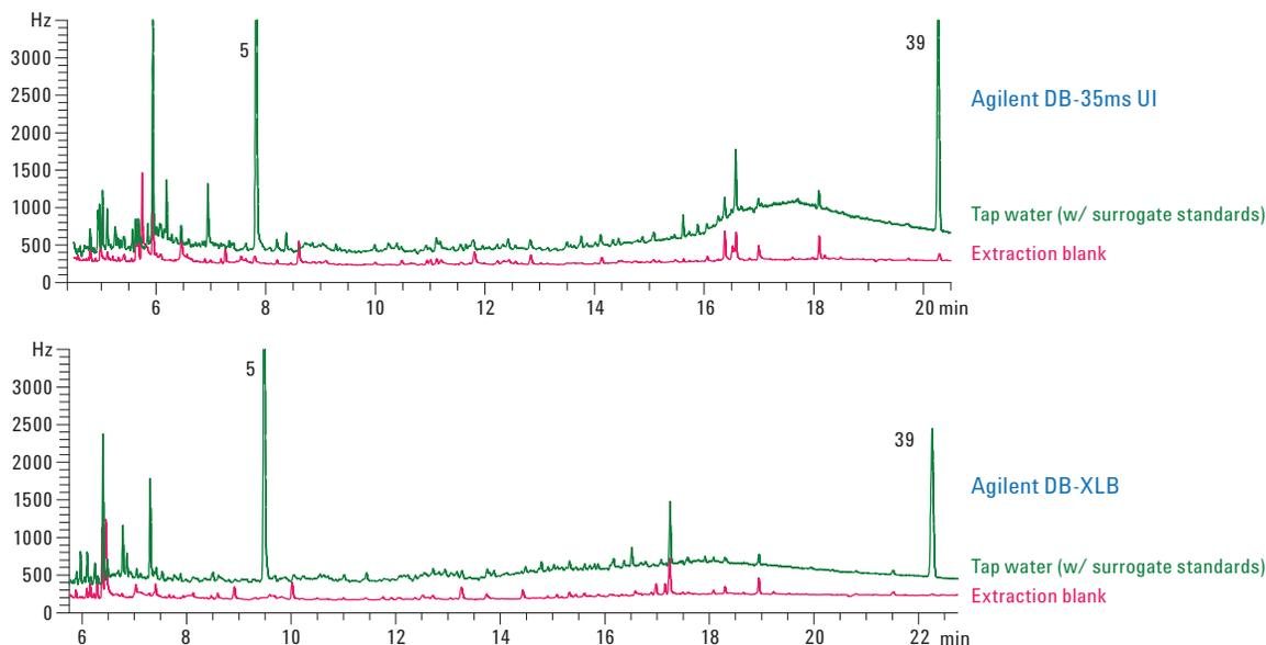
Figure 6. GC/ $\mu$ ECD chromatogram for a tap water sample and extraction blank analyzed using Agilent J&W DB-35ms UI 30 m  $\times$  0.32 mm, 0.25  $\mu$ m column (p/n 123-3832UI) and an Agilent DB-XLB 30 m  $\times$  0.32 mm, 0.5  $\mu$ m column (p/n 123-1236). These samples were prepared and extracted according to the sample preparation procedure detailed in Figure 1. Chromatographic conditions are listed in Table 1.
