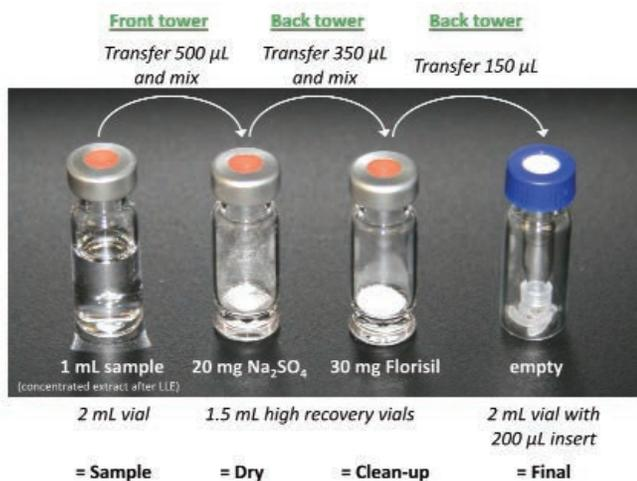
Figure 2. Picture of 2-mL vials during different clean-up steps on Work Bench
