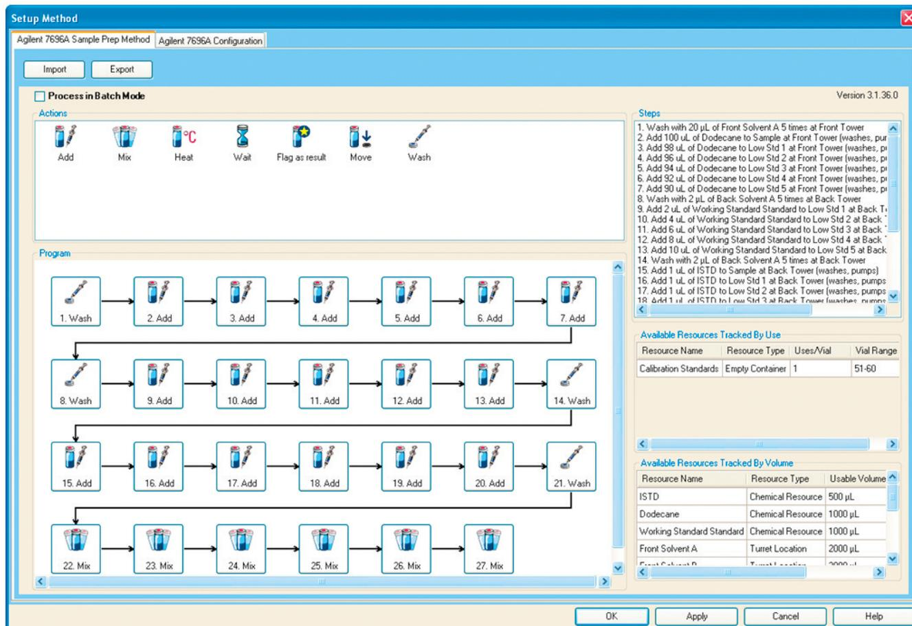
Figure 2. Agilent WorkBench method IP585\_Low.M for preparing five low level calibration standards. Each of the method's steps were built using a "drop-and-drag" graphic user interface.
