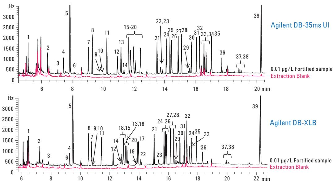
Figure 5. GC/ $\mu$ ECD chromatogram for a 0.01  $\mu$ g/L fortified water sample and extraction blank analyzed using Agilent J&W DB-35ms UI 30 m  $\times$  0.32 mm, 0.25  $\mu$ m column (p/n 123-3832UI) and an Agilent DB-XLB 30 m  $\times$  0.32 mm, 0.5  $\mu$ m column (p/n 123-1236). These samples were prepared and extracted according to the sample preparation procedure detailed in Figure 1. Chromatographic conditions are listed in Table 1.
