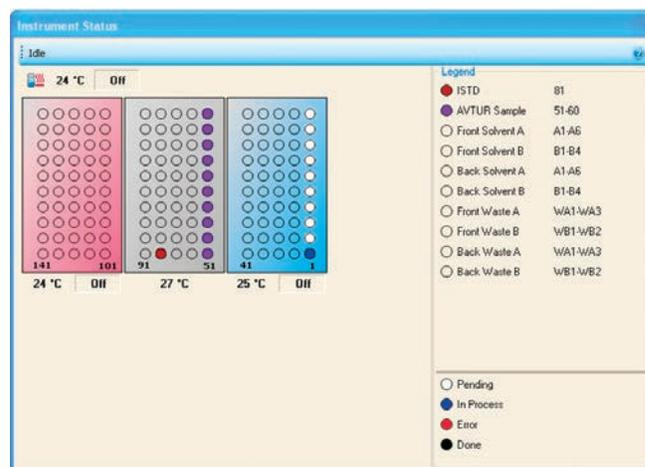
Figure 3. Agilent WorkBench resource layout for the automated preparation of 10 jet fuel samples. The empty vials in positions 1 to 10 will contain the final 100  $\mu\text{L}$  of each jet fuel sample and internal standard after the automated preparation is complete.
