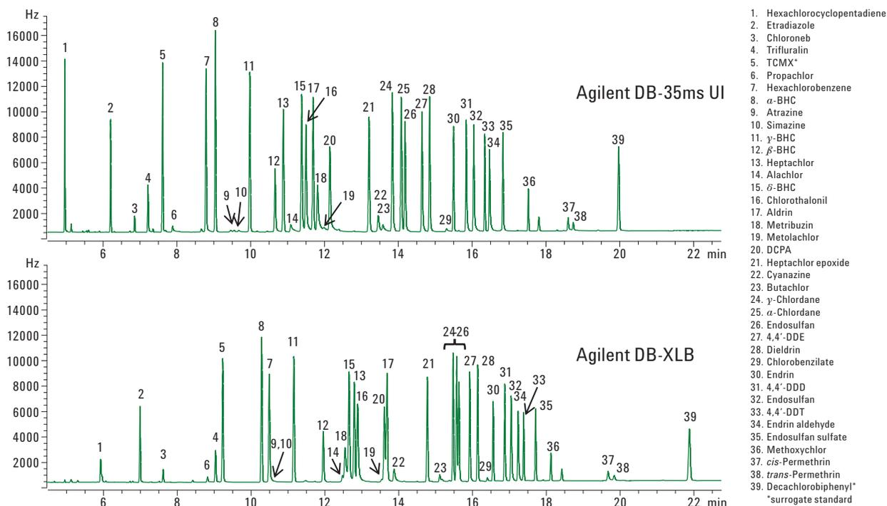
Figure 2. GC/ $\mu$ ECD chromatogram of a 50 ng/mL pesticide standard analyzed on an Agilent J&W DB-35ms UI 30 m  $\times$  0.32 mm, 0.25  $\mu$ m column (p/n 123-3832UI) and DB-XLB 30 m  $\times$  0.32 mm, 0.5  $\mu$ m column (p/n 123-1236). This standard was prepared in ethyl acetate using an Agilent 7696A Sample Prep WorkBench. Chromatographic conditions are listed in Table 1.
