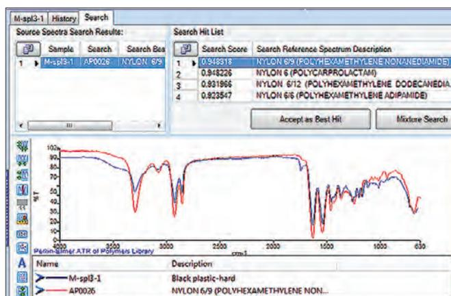
Figure 9. Sample 1 identified as Nylon base material.
