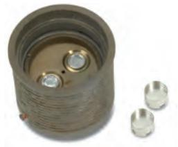
Figure 2. The double-furnace design pictured on the right allows very fast cooling and heating required for isothermal crystallization studies.
