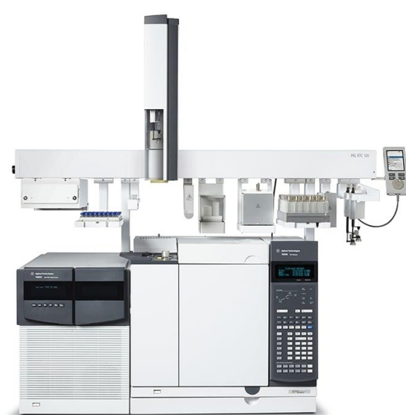
PAL RTC rail system, combined with an Agilent 7890B GC and 5977B High GC/MSD.
