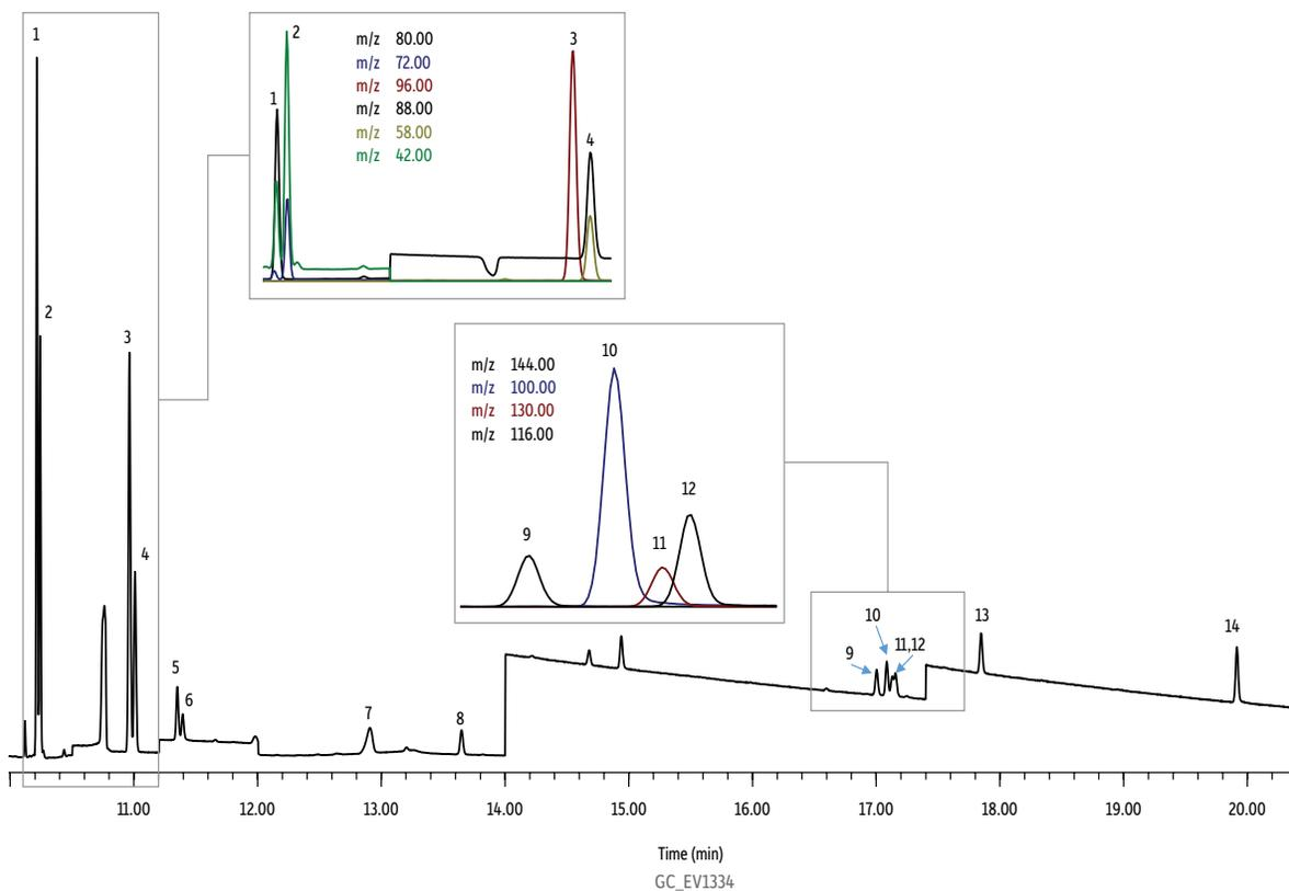
**Column** Rxi®-5Sil MS, 30 m, 0.25 mm ID, 1.00 µm (cat.# 13653) using Rxi® guard column 10 m, 0.53 mm ID (cat.# 10073) with SGE® µ-union
