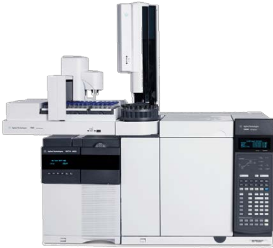
Agilent 7890B GC equipped with 7650A autosampler and 5977A MSD operating in EI mode at 70 eV - FID detector Scan speed 20,000 amu/s Etune option
