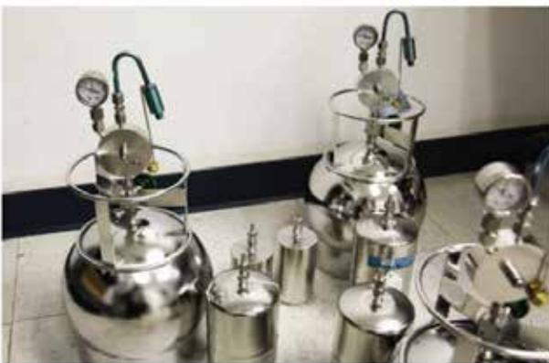
**Figure 2** 6L Classical sampling canisters collecting 24 hour samples along side smaller 0.45L and 1.4L HDS's.
