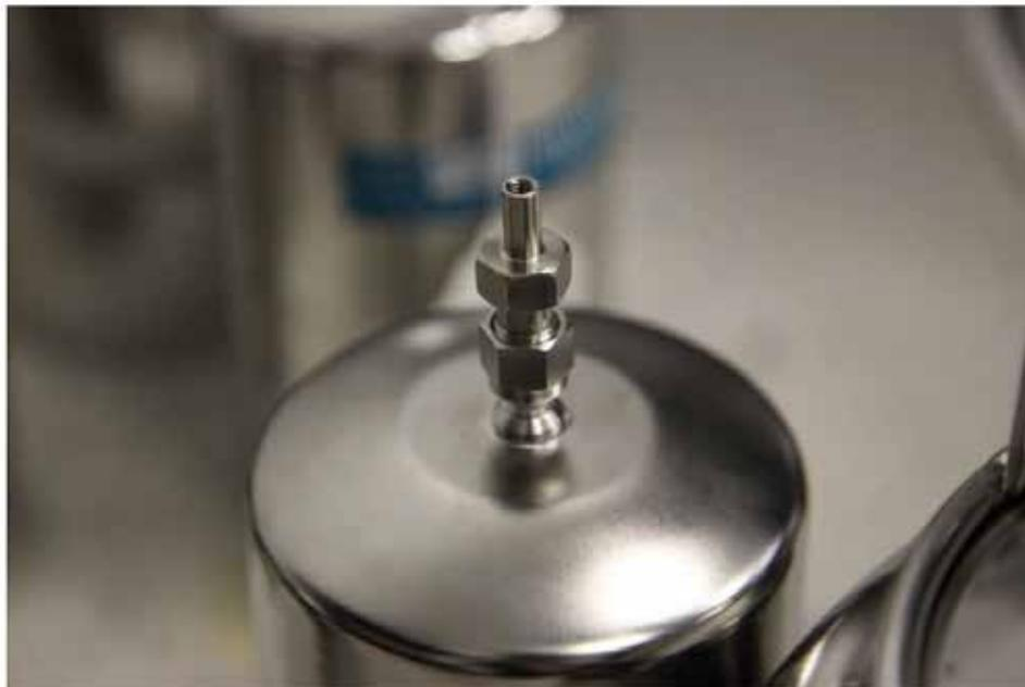
**Figure 3** Close up view of the HDS inlet orifice built right into the 1.4L canister valve.
