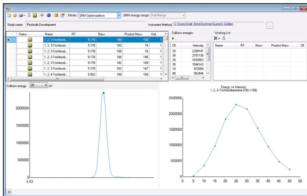
Figure 2. Collision energy optimization curve for the  $m/z$  180  $\rightarrow$  109 transition of 1, 2, 3-Trichloroethane, showing an optimum collision energy of 25 eV. At this point in the process, the optimized SRM transitions can be exported to your instrument method.
