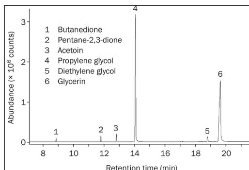
**Figure 4:** Analysis of an e-cigarette impurities mix using TD–GC–MS, showing no co-elution of low-level compounds with matrix components (#4 and #6).
