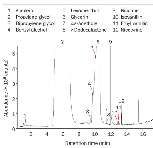
**Figure 5:** TD–GC–MS analysis of vapour from an e-cigarette loaded with a ‘tobacco-flavoured’ e-liquid, indicating major components and some trace-level components with regulatory or organoleptic relevance.
