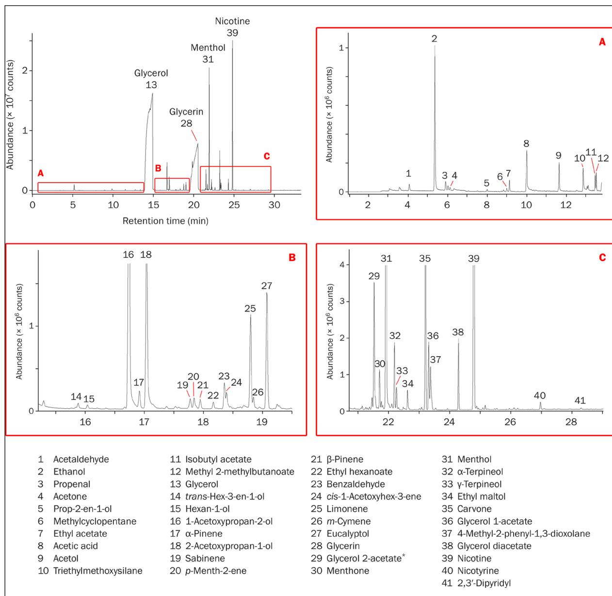
**Figure 6:** TD-GC-MS analysis of vapour from an e-cigarette loaded with a 'menthol and blueberry' flavour e-liquid, indicating major components and a selection of lower-level components (some with regulatory or organoleptic relevance). \* = Identity tentative.
