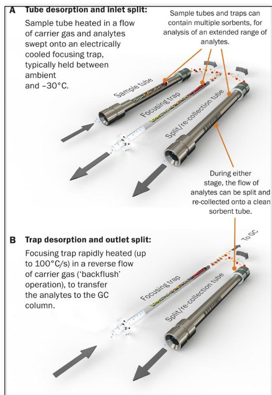
Figure 1: How two-stage thermal desorption works.
