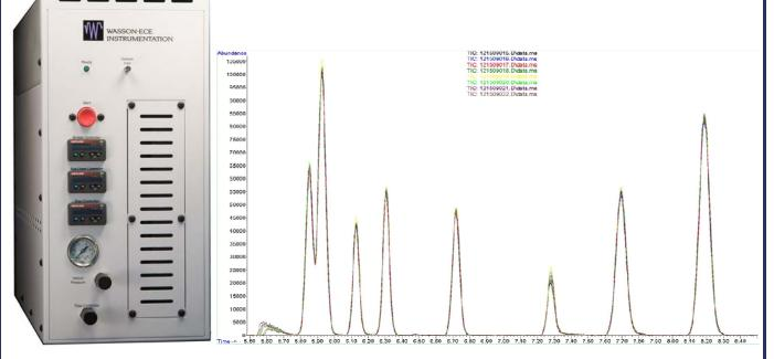
Figure 2: VOC concentration system with repeatability of < 5% on the GC/MSD at 10-999 mL load volumes.
