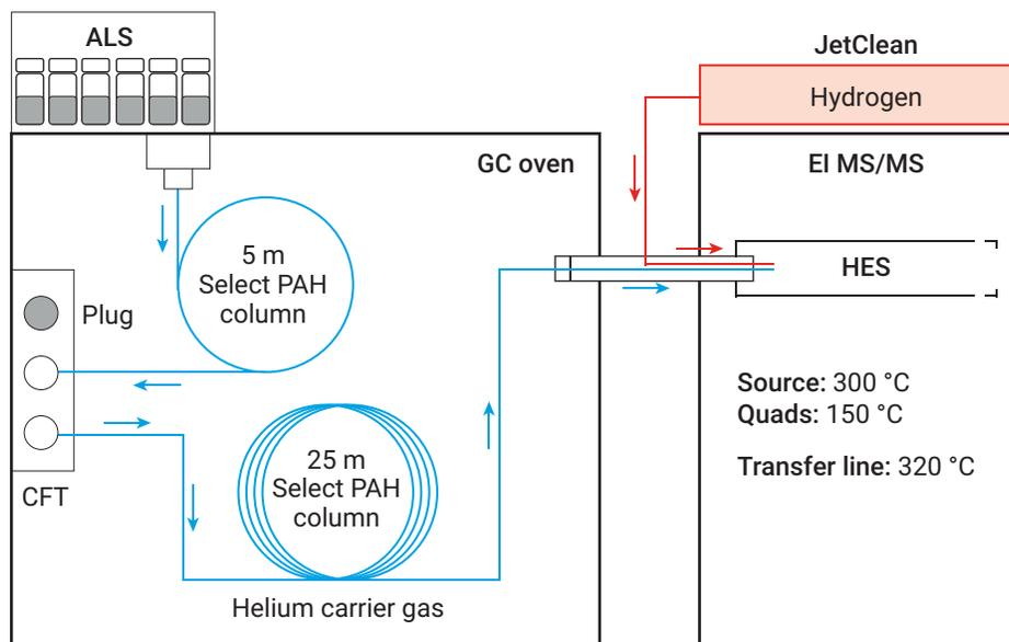
Figure 2. GC/MS/MS in electron ionization (EI) mode configured with BF and JetClean. Arrows indicate direction of helium carrier gas flow. CFT purged 3-way splitter is used to configure the two columns for BF. The JetClean self-cleaning ion source is configured to the MSD in Acquire and Clean mode to allow 0.33 mL/min of hydrogen flow to the source. HES = high efficiency source. CFT = Capillary Flow Technology.
