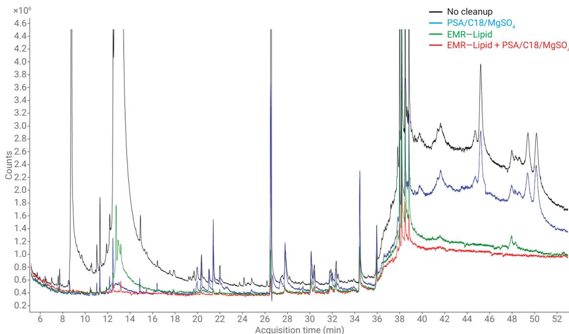
**Figure 3.** Pumpkin seed oil extracts with different cleanup procedures. MS scan range  $m/z$  40 to 1,050. Black: no cleanup. Blue: PSA/C18/MgSO<sub>4</sub> cleanup. Green: EMR–Lipid cleanup. Red: EMR–Lipid with an additional PSA/C18/MgSO<sub>4</sub> cleanup.
