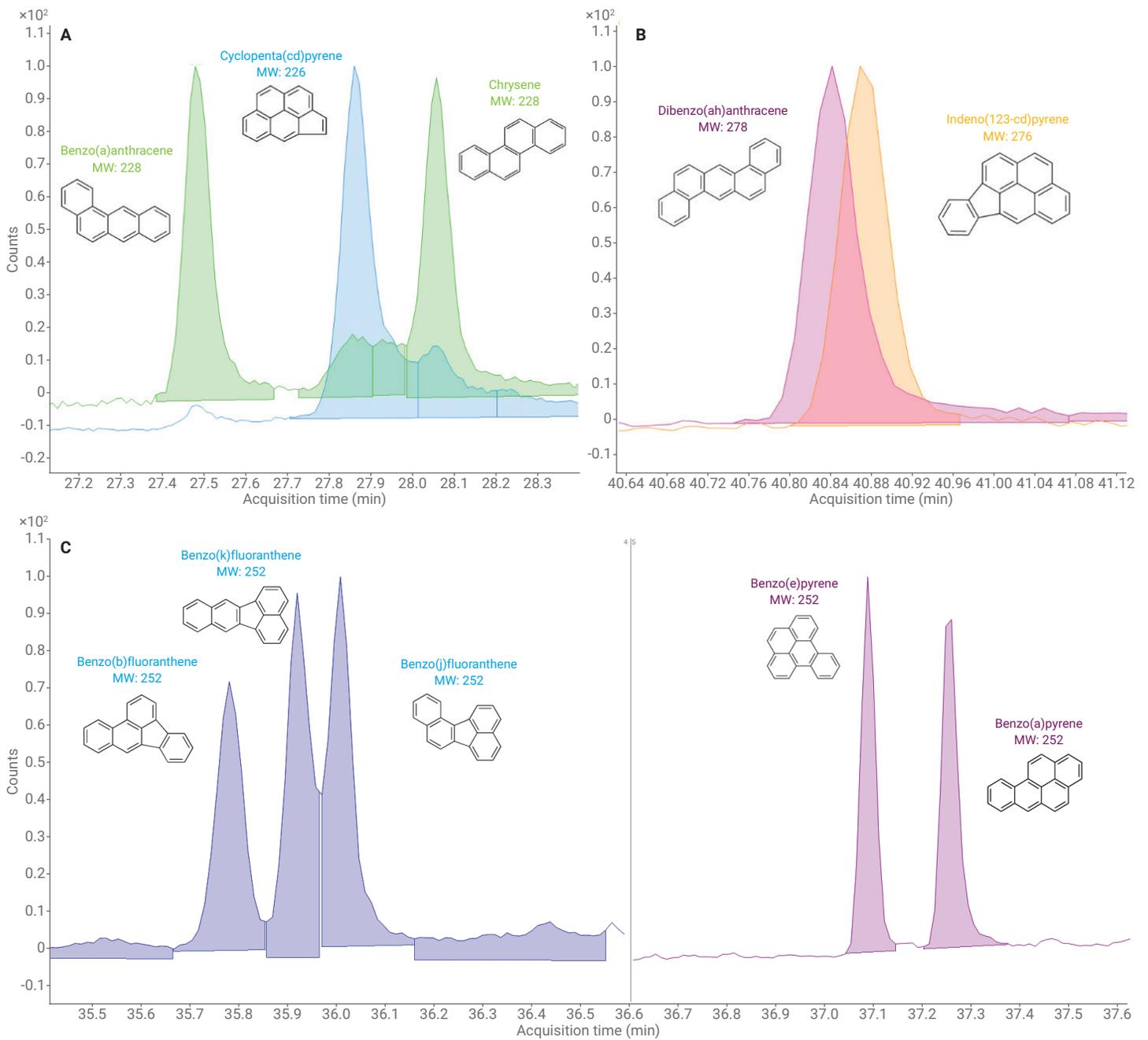
**Figure 5.** GC/MS/MS MRM chromatograms of pumpkin seed oil spiked with 5 ng/g PAHs (A-E). Collision energy of 50 eV. Quantifier transitions  $[M]^+ \rightarrow [M]^+$  are plotted, where M represents molecular mass.
