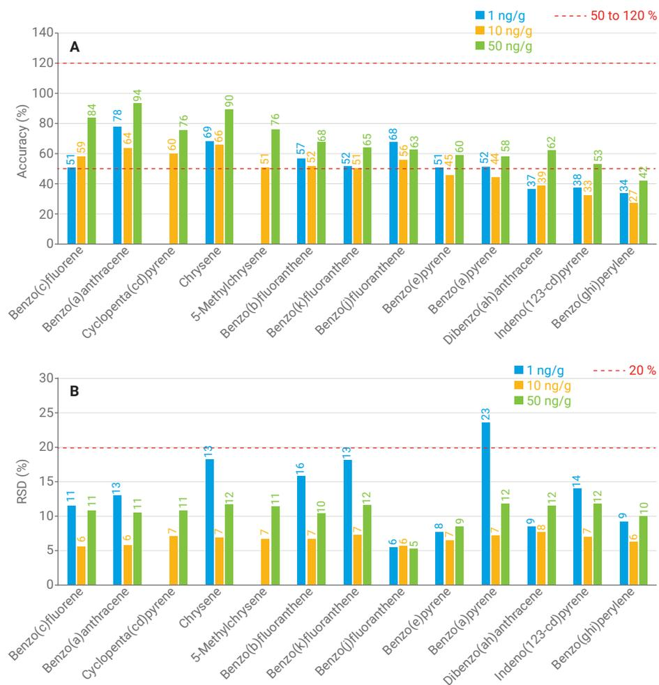
**Figure 8.** Recovery (A) and RSD (B) of pumpkin seed oil spiked with 1 ng/g (blue), 10 ng/g (yellow), and 50 ng/g (green) PAH standards. n=6. Analytes are plotted in order of increasing retention time.
