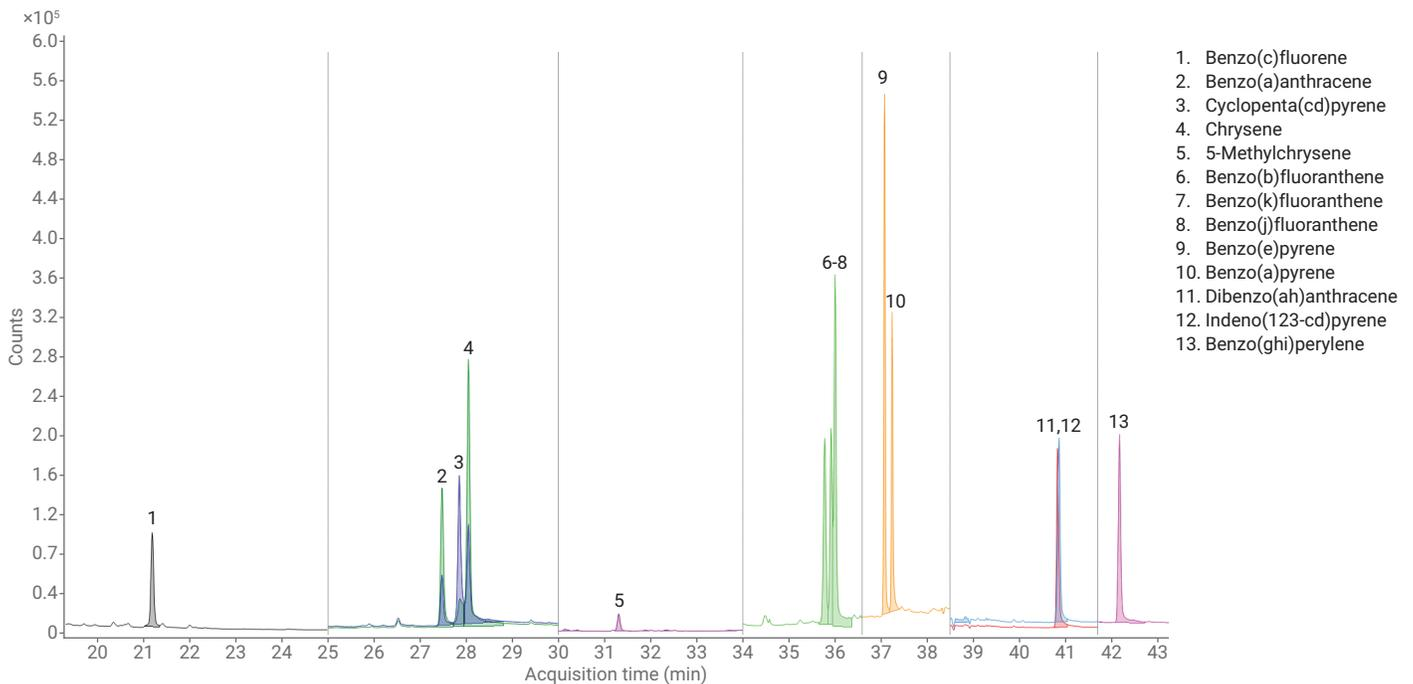
**Figure 4.** MRM TIC of quantifier ion from matrix-matched calibration of pumpkin seed oil spiked with 50 ng/g PAH. Collision energy of 50 eV. Quantifier transitions  $[M]^+ \rightarrow [M]^+$  are plotted, where M represents molecular mass.
