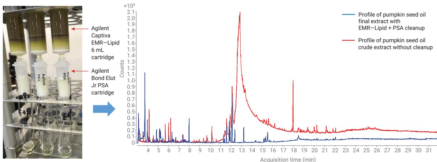
**Figure 3.** Agilent Captiva EMR-Lipid hyphenated with Bond Elut Jr PSA provides efficient cleanup for pumpkin seed oil matrix, with demonstration of attached cartridges (left) and a GC/MS full scan for cleanup efficiency (right).
