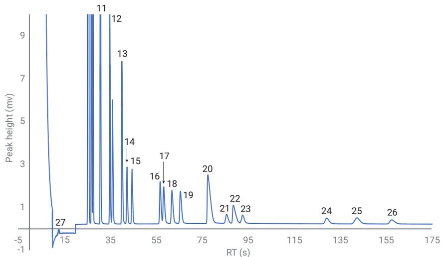
Figure 3. standard gas (simulated RGA) on Al<sub>2</sub>O<sub>3</sub> BF2D channel.
