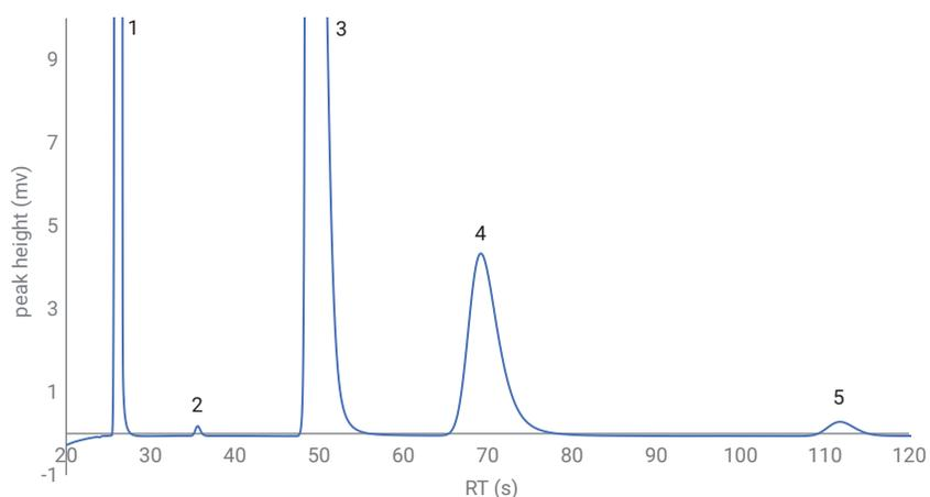
Figure 1. standard gas (simulated RGA) on MS5A channel.
