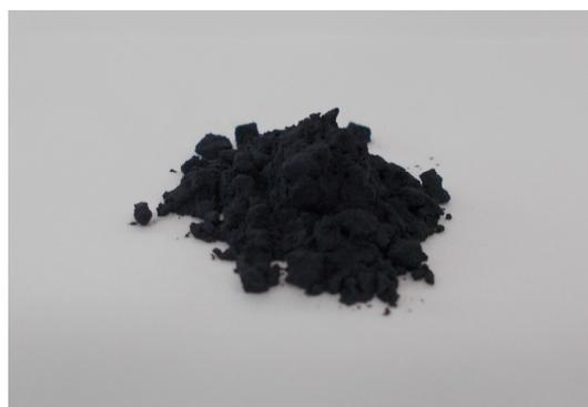
Fig. 2 Lithium Cobalt Oxide
