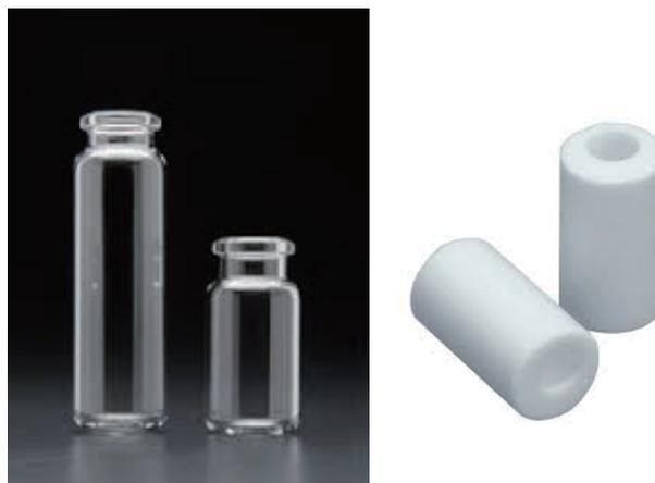
Figure 2. Headspace vial and monotrapp
